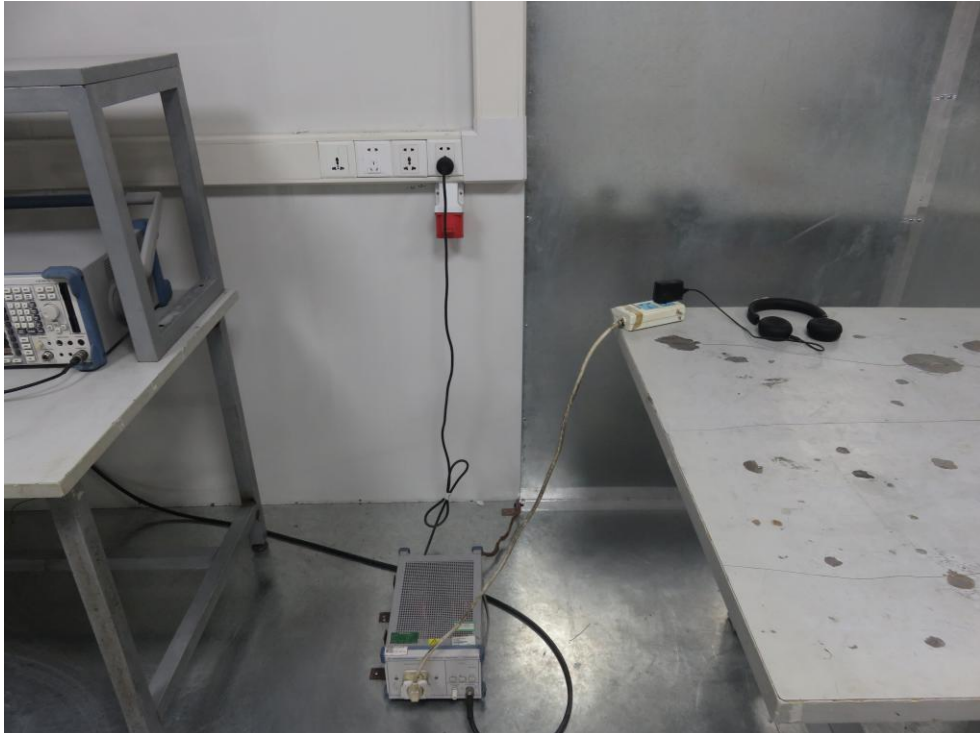
Photo of Conducted Emission Measurement
