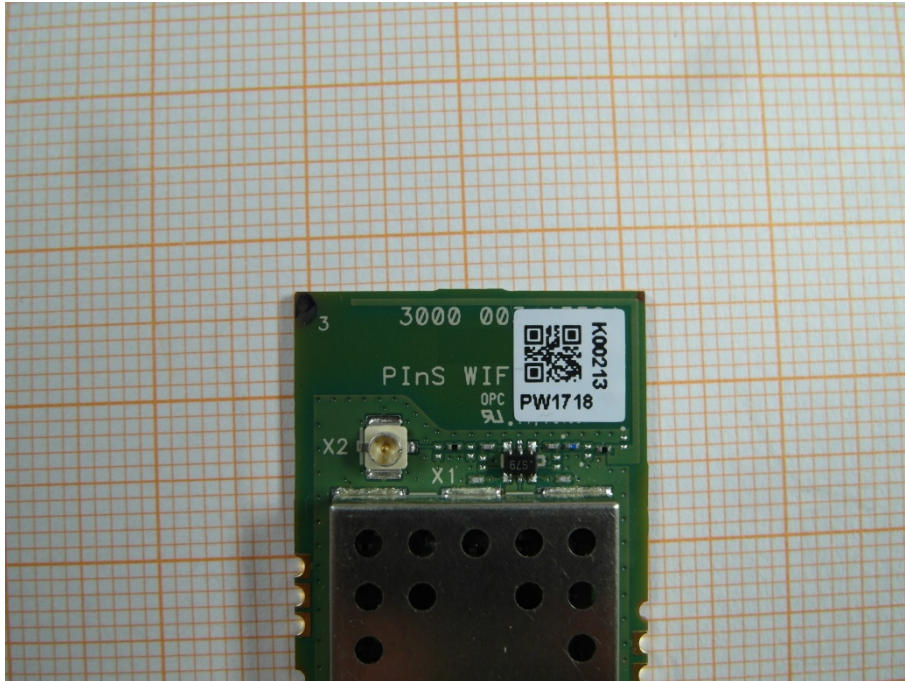
Photo 3: Internal antenna, antenna switch + antenna port for external antenna
