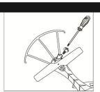
Attack the X-Guards to the end of each rotor using the included small screwdriver. Place the small plastic round tabs into the holes on each rotor arm. Firmly tighten the screws in place, making sure that the X-Guards are facing out and that the center bar of the guard is lined up with the arm of the rotor.
