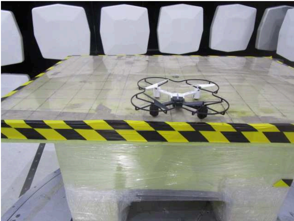
Up to 1GHz (EUT was placed at the centre of the turntable)
