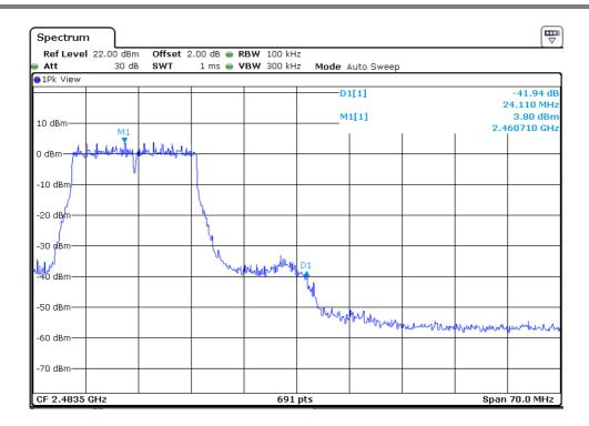
802.11n-HT20 Channel 01 (2412MHz) Reference Level: 4.39dBm
