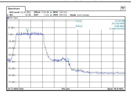
802.11n-HT20 Channel 01 (2412MHz) Reference Level: 4.39dBm
