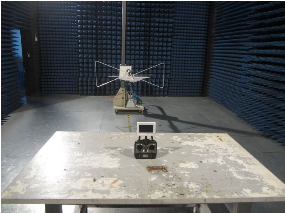
Setup for radiated emission
