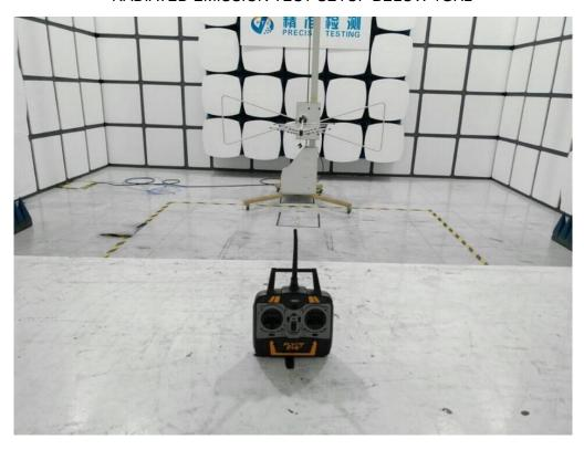
RADIATED EMISSION TEST SETUP ABOVE 1GHz
