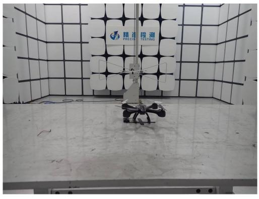
RADIATED EMISSION TEST SETUP ABOVE 1GHz
