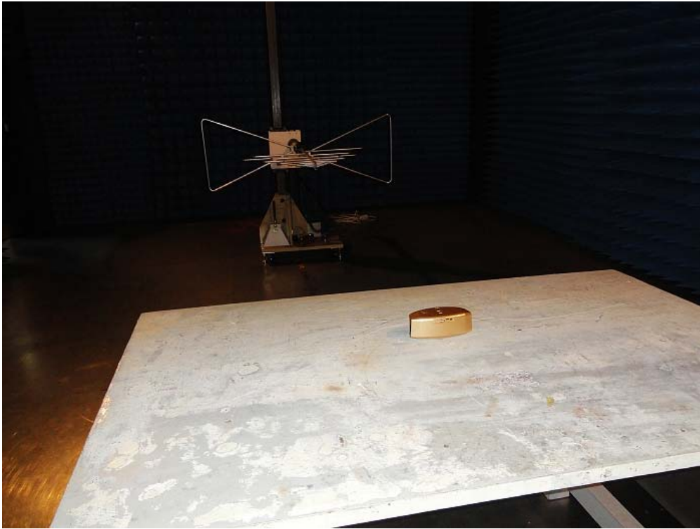
Radiated Emission Test Setup:
