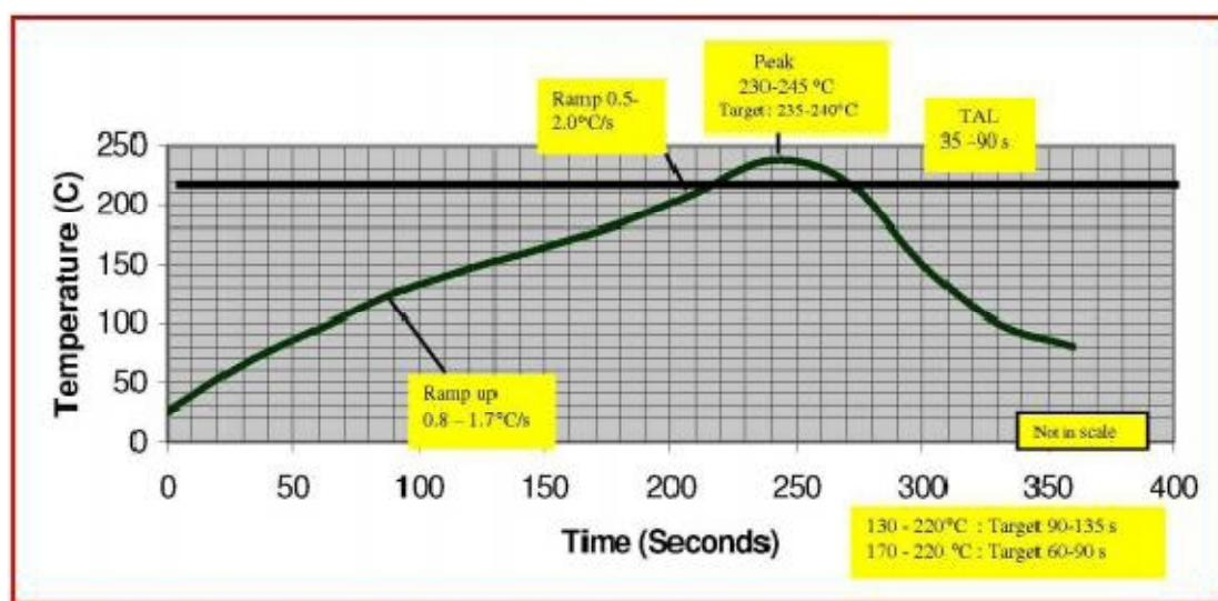
Note: as shown in the above figure, it is based on the SAC305 lead-free tin paste (3% silver, 0.5% copper). Alpha OM-338 lead-free cleaning-free flux is recommended. This figure is mainly used for guidance. The entire process time is subject to thermal pad number of assembly board and device Intensity.
