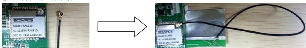
The antenna is installed inside the host unit and the final user can not install the antenna themselves. The module and antenna are installed with a distance over 20cm from the user during use.
