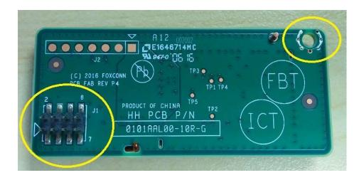
The Qolsys Z-WaveAH Plus Module operates at 919.8 / 921.4 MHz with an output power set at 0 dBm with trace and filter loss is approx.. 1.3 dbi. Data and protocol specifications are beyond the scope of this document. Please contact Qolsys for the technical specifications.
