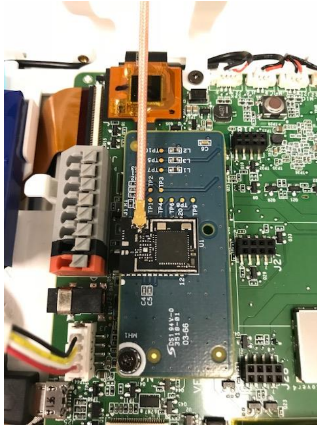
Figure 3: Test Setup for conducted measurements at temporary u.fl connector – EUT Qolsys Zigbee Radio Card QS-ZB – integrated in QS-IQPANEL2 auxiliary host – Detail
