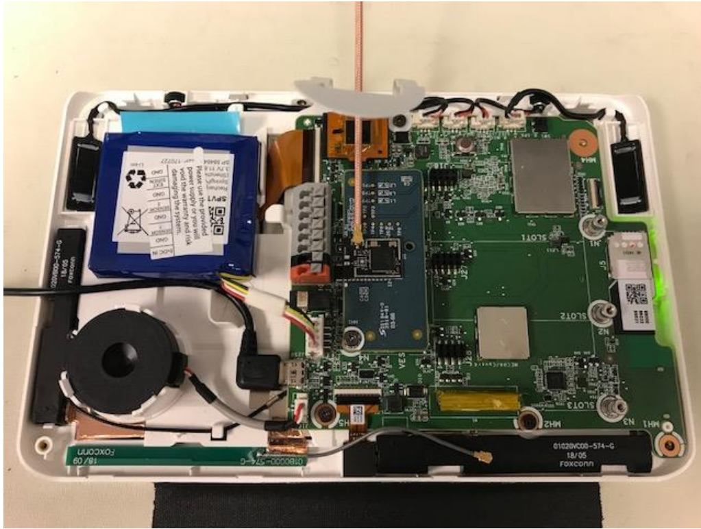
Figure 2: Test Setup for conducted measurements at temporary u.fl connector – EUT Qolsys Zigbee Radio Card QS-ZB – integrated in QS-IQPANEL2 auxiliary host
