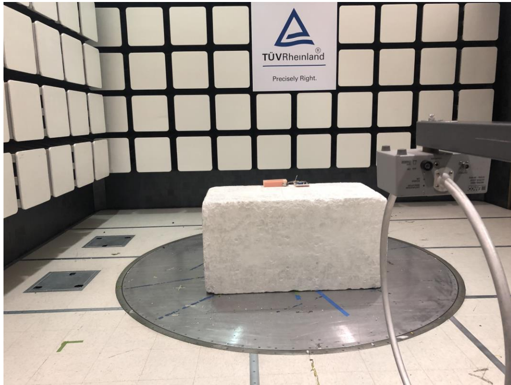
Figure 5: Test Setup for 30 MHz to 1 GHz (Front View – Antenna 90°)
