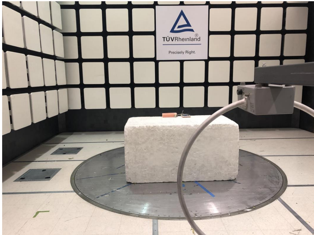
Figure 4: Test Setup for 30 MHz to 1 GHz (Front View – Antenna 0°)
