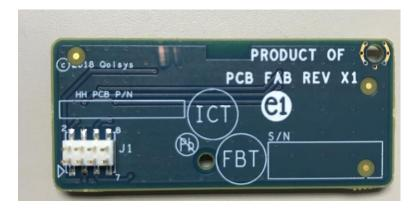
The Qolsys Zigbee Card operates around 2.4GHz with an output power up to +10dBm. Data and protocol specifications are beyond the scope of this document. Please contact Qolsys for the technical specifications.
