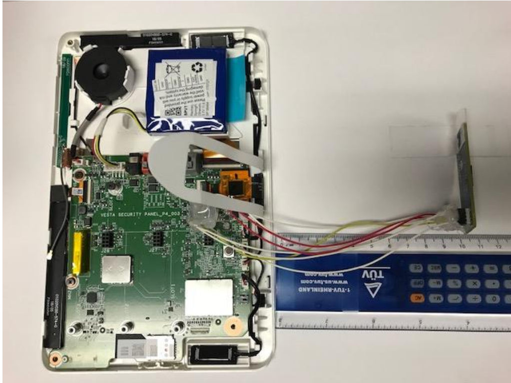
Figure 5: Picture Qolsys Zigbee Radio Card – Radiated Test Sample - Connected to auxiliary host QS-IQPANEL2 via wire extension
