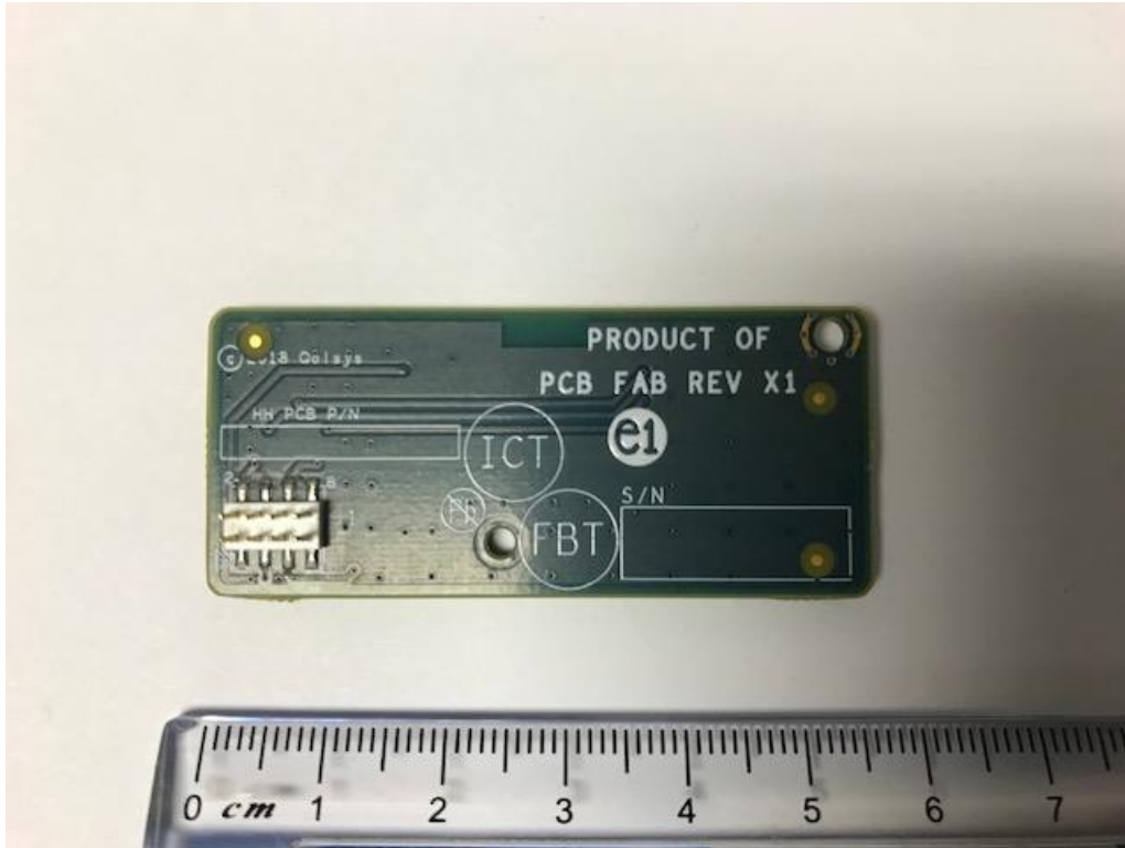
Figure 4: Internal Picture Qolsys Zigbee Radio Card - Conducted test sample - Rear
