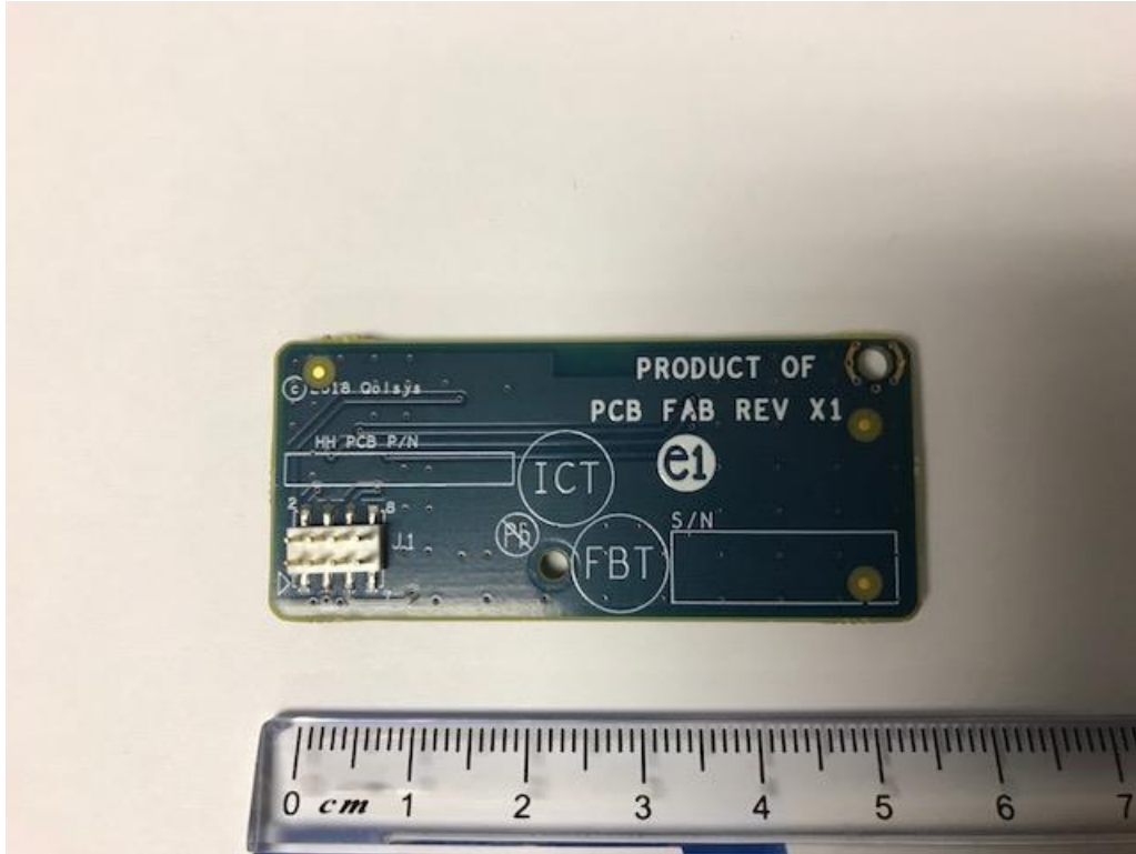
Figure 2: Internal Picture Qolsys Zigbee Radio Card - QS-ZB – Radiated Sample - Rear
