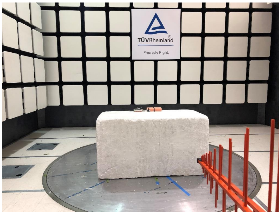
Figure 8 - Radiated Emissions 30MHz - 1 GHz rear - EUT Horizontal
