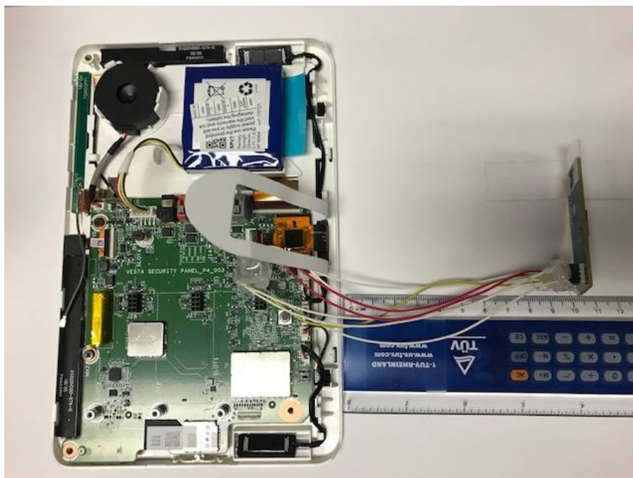
Figure 4: External Photo Qolsys Zigbee Radio Card QS-ZB– Host Unit – Detail – EUT module separation > 10cm
