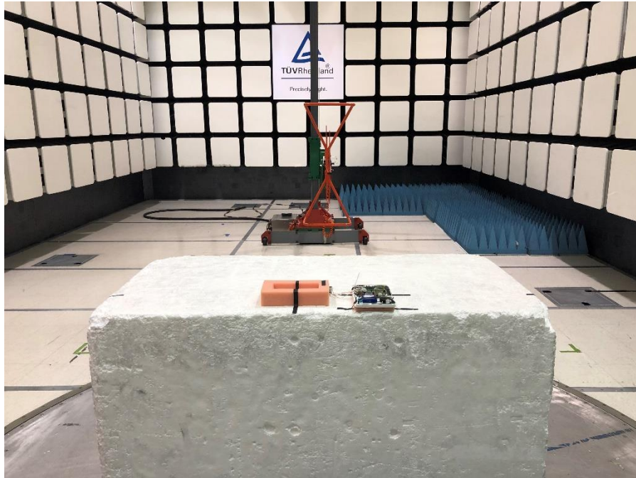
Figure 7 - Radiated Emissions Test Setup 30 - 1000 MHz - Front
