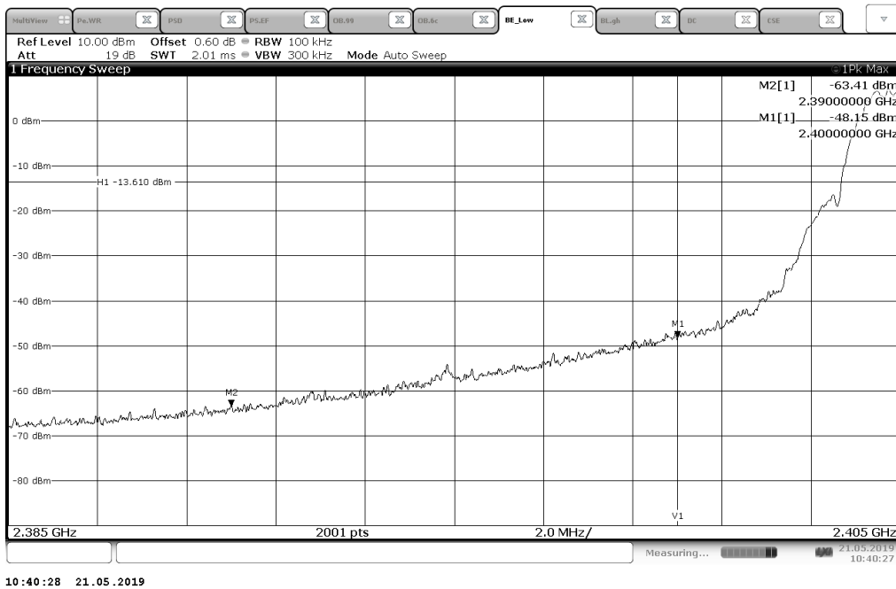
Figure 16: Lower Band Edge – IEEE 802.15.4 - ZIGBEE – 2405 MHz
