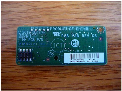
The Qolsys SRF319-4 Module operates at 319.5 MHz with an output power set at 0 dBm with trace and filter loss is approx.. 1.3 dbi. Data and protocol specifications are beyond the scope of this document. Please contact Qolsys for the technical specifications.
