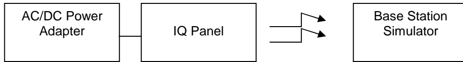
Block Diagram for Radiated Tests
