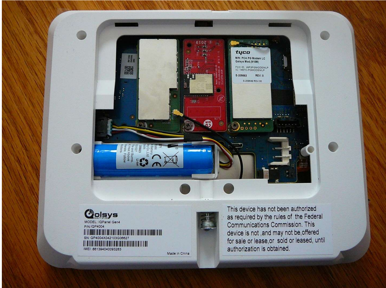
Backside View with Mounting cover removed
