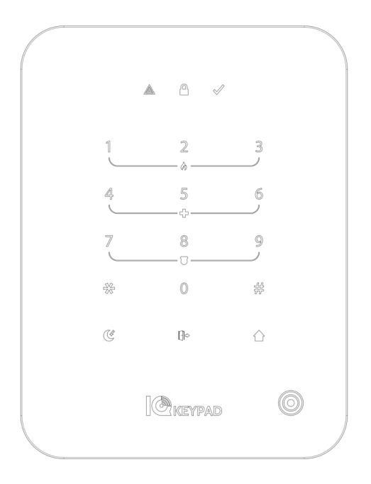
IQ Keypad is a battery powered, capacitive touch keypad for use with compatible IQ4 NS, IQ4 Hub & IQ Panel 4 platforms via the PowerG protocol. It provides an easy and intuitive interface to control basic features of the system. This manual covers both IQ Keypad Prox-PG and IQ Keypad-PG models.
