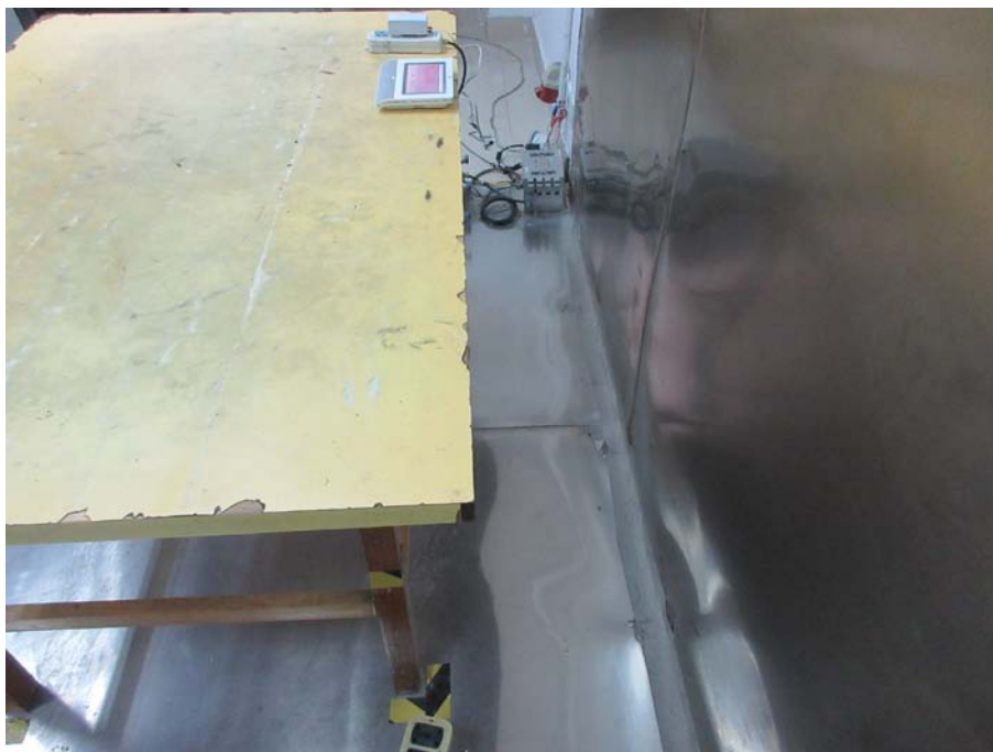
Conducted Emissions Test Setup Side View
