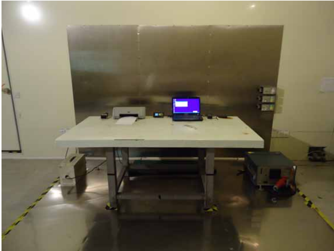
Front View of Conducted Disturbance Measurement
