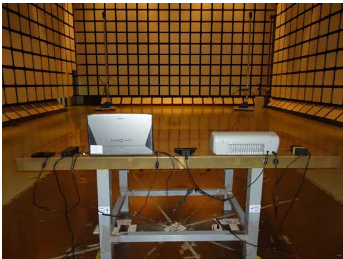
Back View of Radiated Disturbance Measurement
