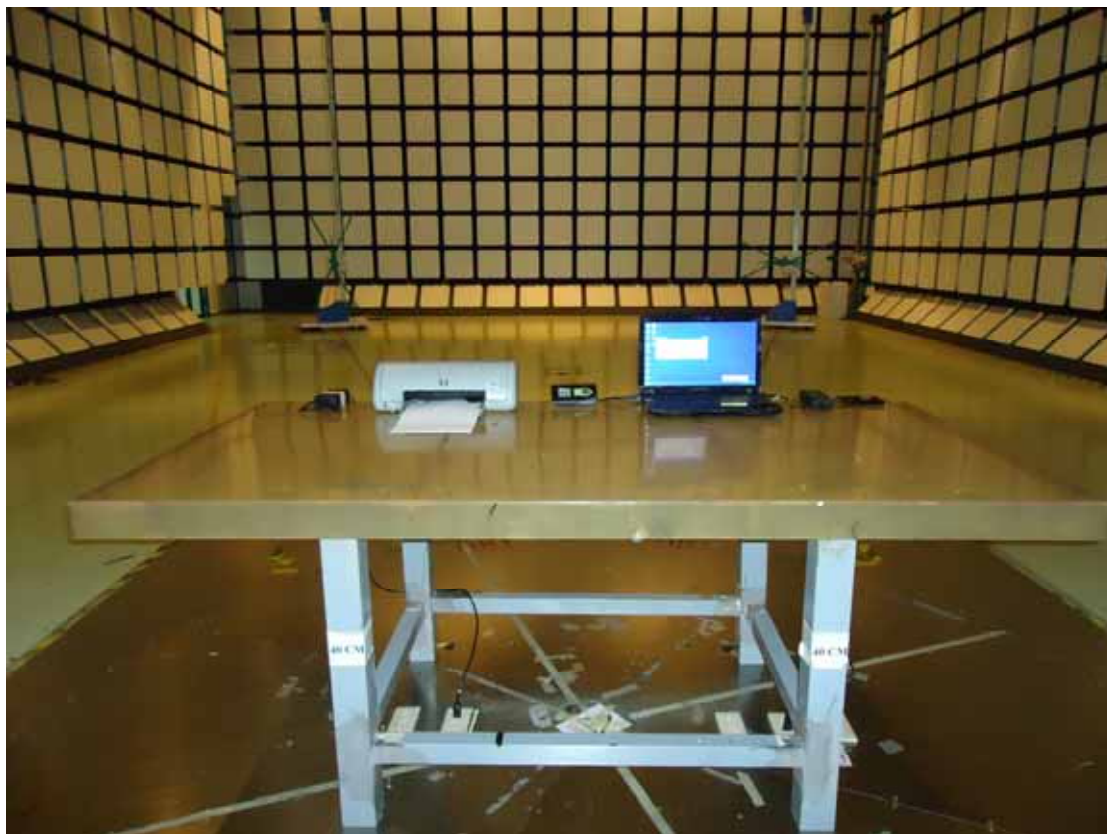
Front View of Radiated Disturbance Measurement
