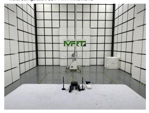
Description: Radiated Spurious Emission Test Setup for Above 1GHz Configuration: EUT + Wi-Fi Antenna #1
