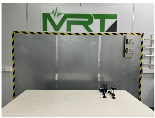
Description: Back View of Conducted Emission Test Setup for Power Port Configuration: EUT + Wi-Fi Antenna #2
