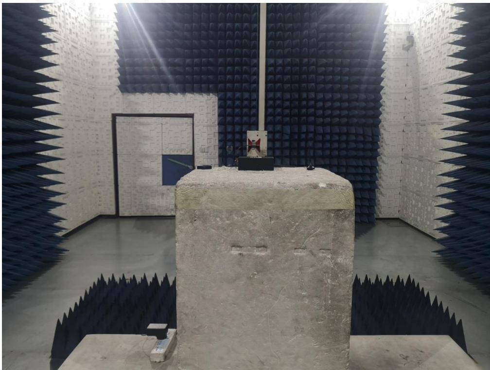
RADIATED SPURIOUS ABOVE 1G EMISSION-Suction Cup Antenna
