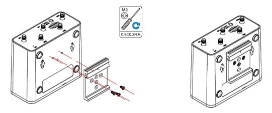
Use 3 pcs of M3\*8 Black cross recessed countersunk head tapping screws to mount the router on the DIN rail, and then hang the DIN rail on the holder. You need to choose a standard holder.
