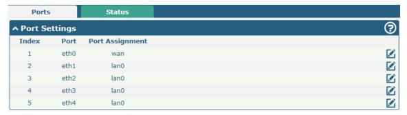
Click the **b**utton on the right-most of eth1 to change the port parameters in the port window that pops up.
