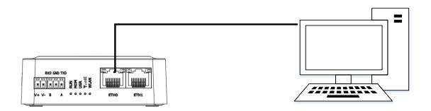
Connect a standard Ethernet cable to the port marked ETH0~ETH1 at the front of the R1511 Router, and connect the other end of the cable to your computer.
