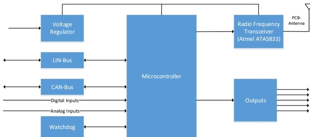
In section 0, the design of the radio frequency transceiver is outlined.
