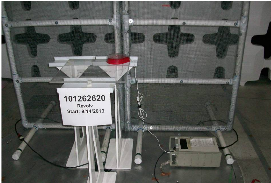
Test Setup – Conducted Emissions (Front View)
