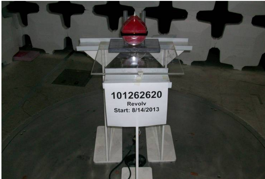
Unintentional Radiated Emissions - Test setup (Front View)
