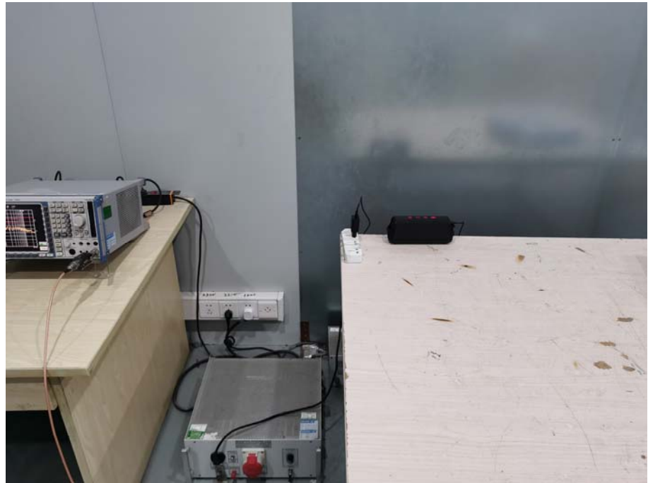
Conducted Emission Test Setup
