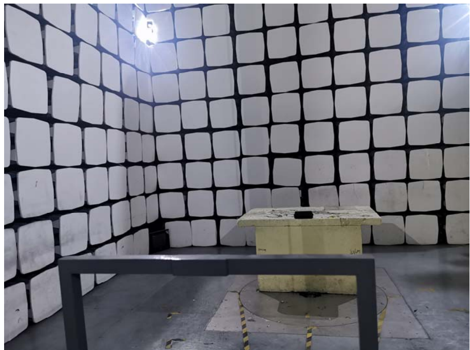
Radiation Emission Test Setup (Below 30MHz)
