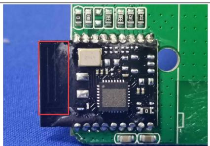
The antenna is PCB antenna. The best case gain of the antenna is 0dBi.
