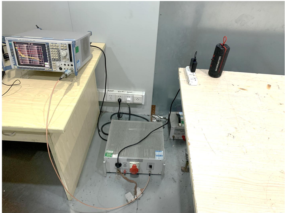
Conducted Emission Test Setup
