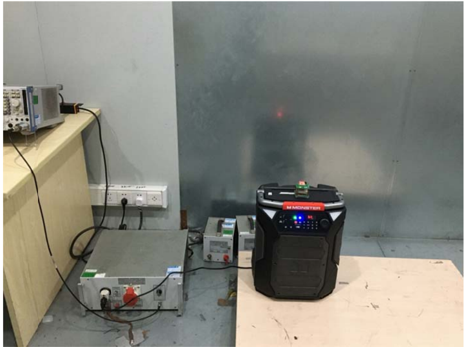
Conducted Emission Test Setup
