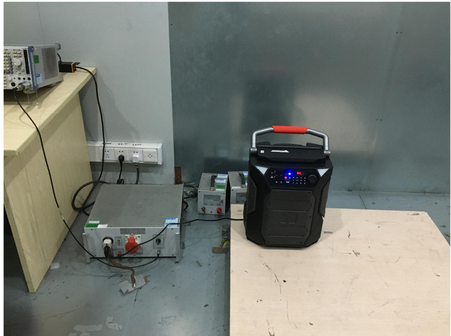
Conducted Emission Test Setup
