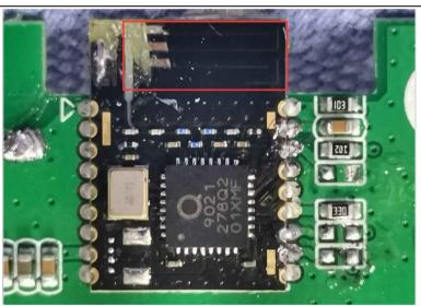
The antenna is PCB antenna. The best case gain of the antenna is 0dBi.
