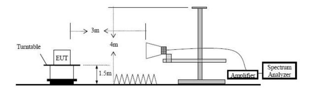
Emission Mask Test set-up.
