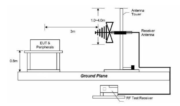
Radiated Emission Test Set-Up, Frequency above 1GHz
