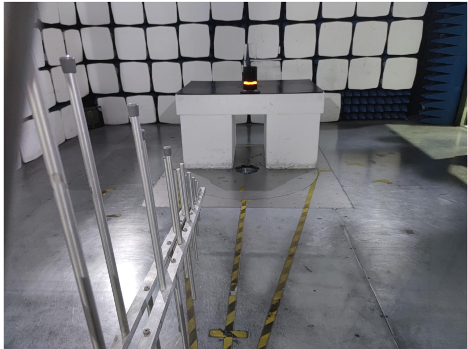
Radiation Emission Test Setup (30MHz to 1GHz)
