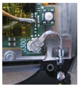
Coax cable feed to monopole antenna molded into the watch band.
