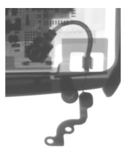
X-Ray shows coax feed and antenna element molded into watch band.
