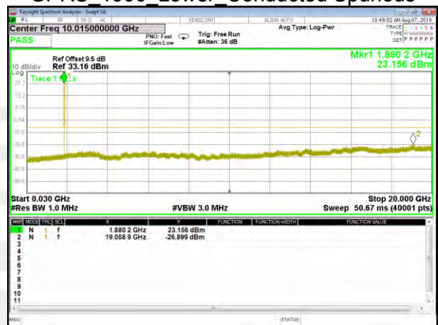
GPRS 1900 Middle Conducted Spurious
