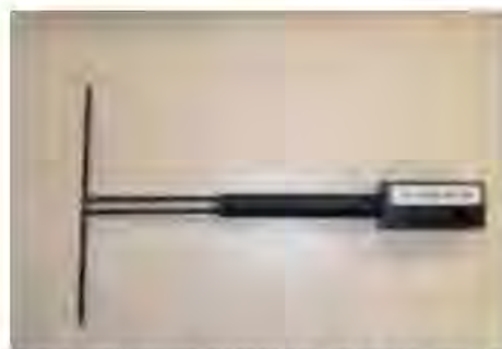
Figure 1 – Satimo COMOSAR Validation Dipole
