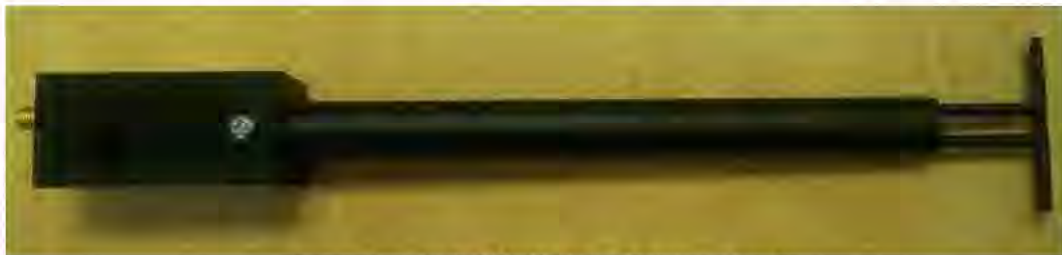
Figure 1 – MVG COMOSAR Validation Dipole
