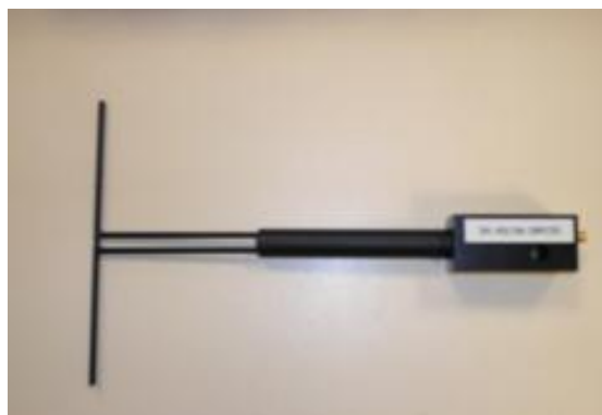
Figure 1 – MVG COMOSAR Validation Dipole
