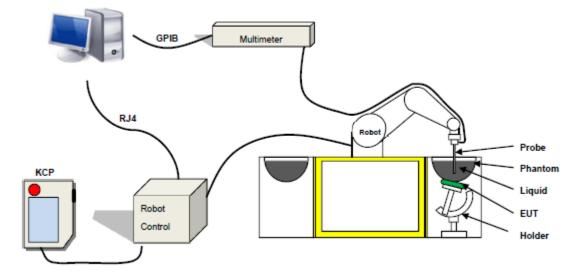
Comosar is a system that is able to determine the SAR distribution inside a phantom of human being according to different standards. The Comosar system consists of the following items:
