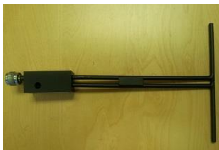
Figure 1 – MVG COMOSAR Validation Dipole
