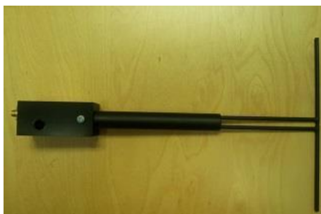
Figure 1 – MVG COMOSAR Validation Dipole
