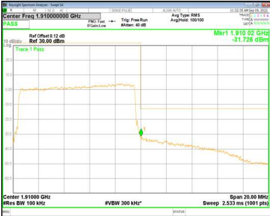
Band2 QPSK BW=15MHz Channel=18675 RB Size=75 Position=#0
