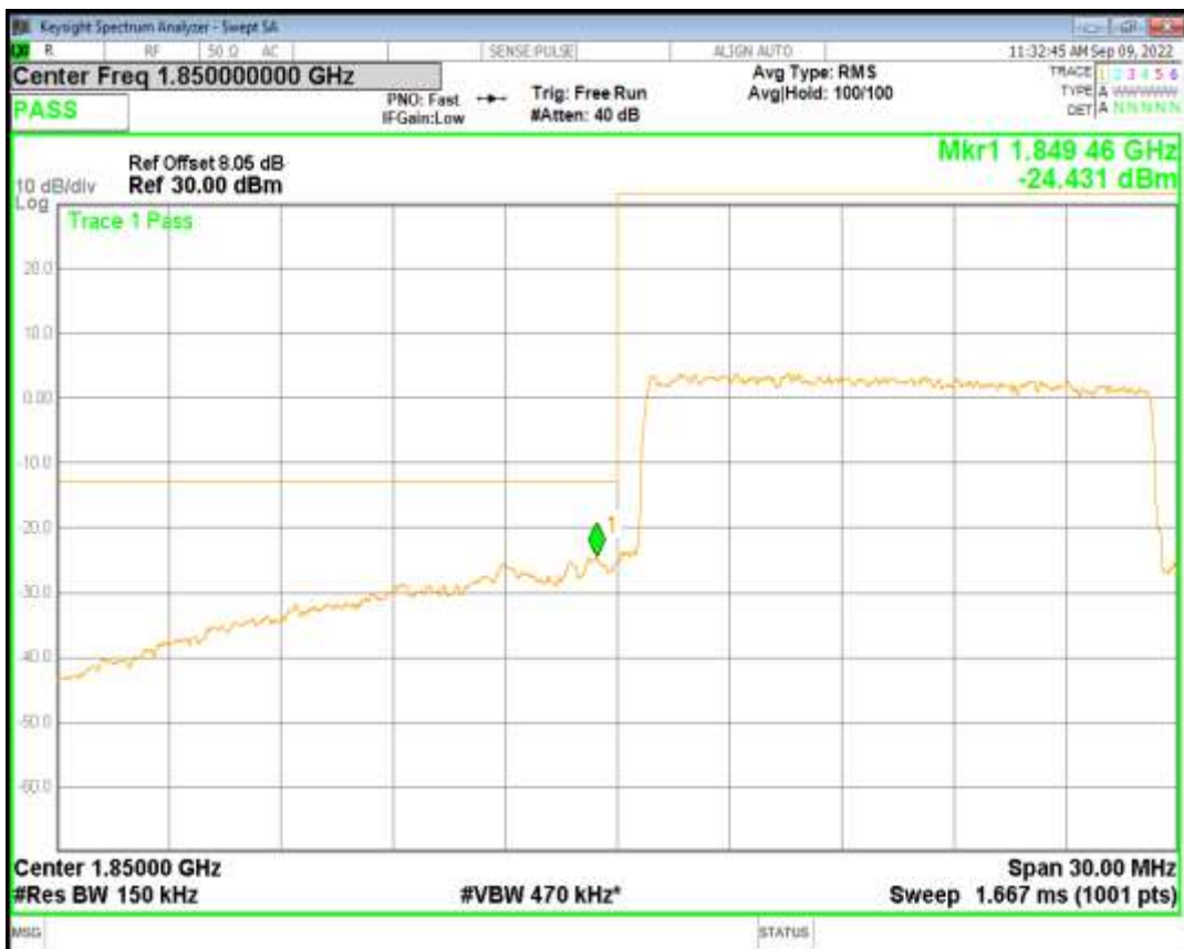
Band2 QAM16 BW=15MHz Channel=18675 RB Size=75 Position=#0
