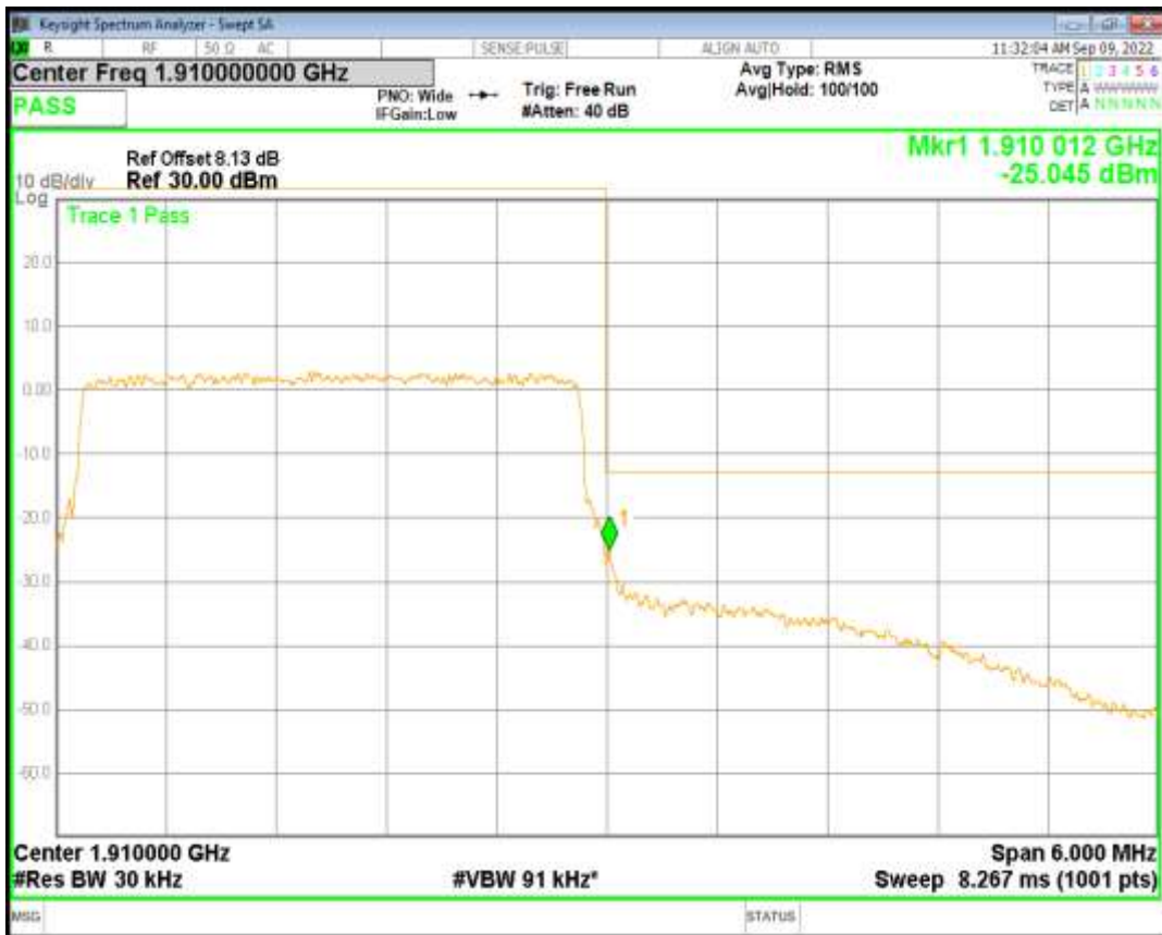
Band2 QPSK BW=5MHz Channel=18625 RB Size=25 Position=#0
