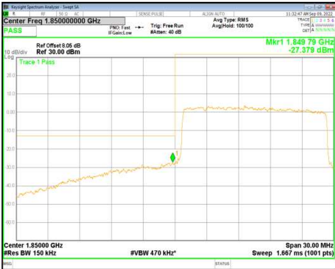
Band2 QPSK BW=15MHz Channel=19125 RB Size=75 Position=#0
