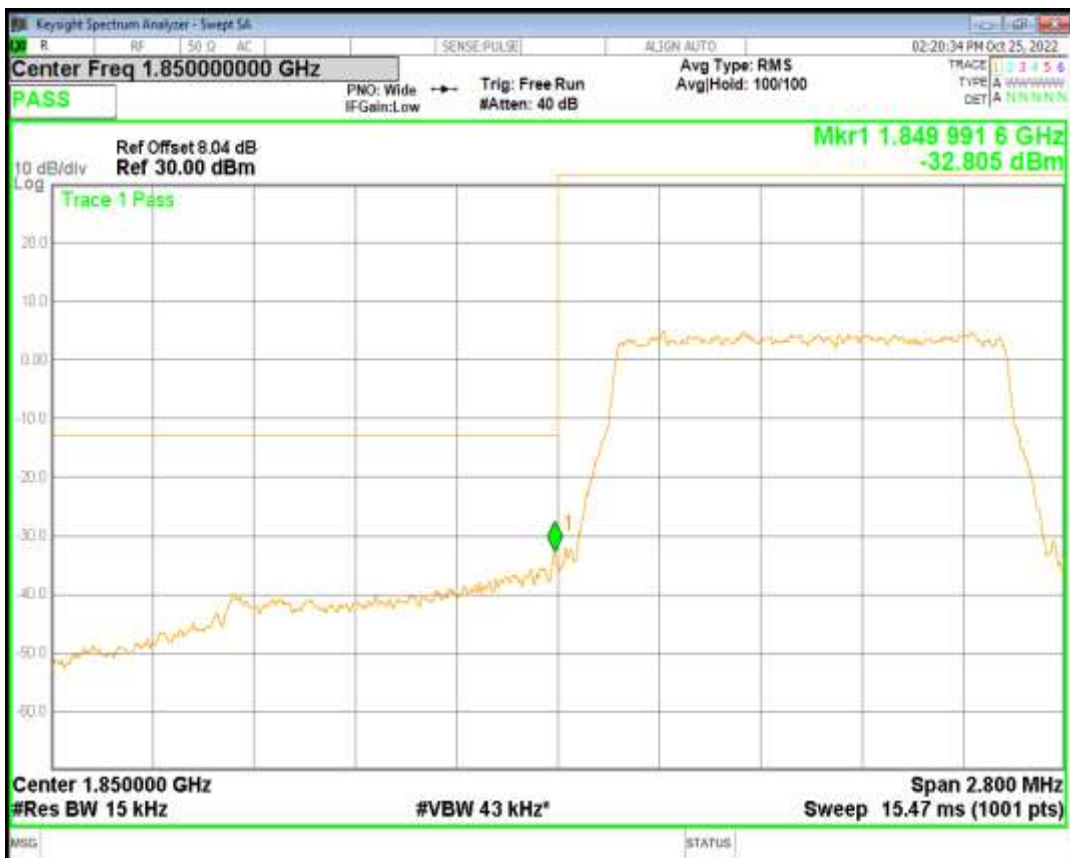
Band25 QAM16 BW=1.4MHz Channel=26047 RB Size=6 Position=#0
