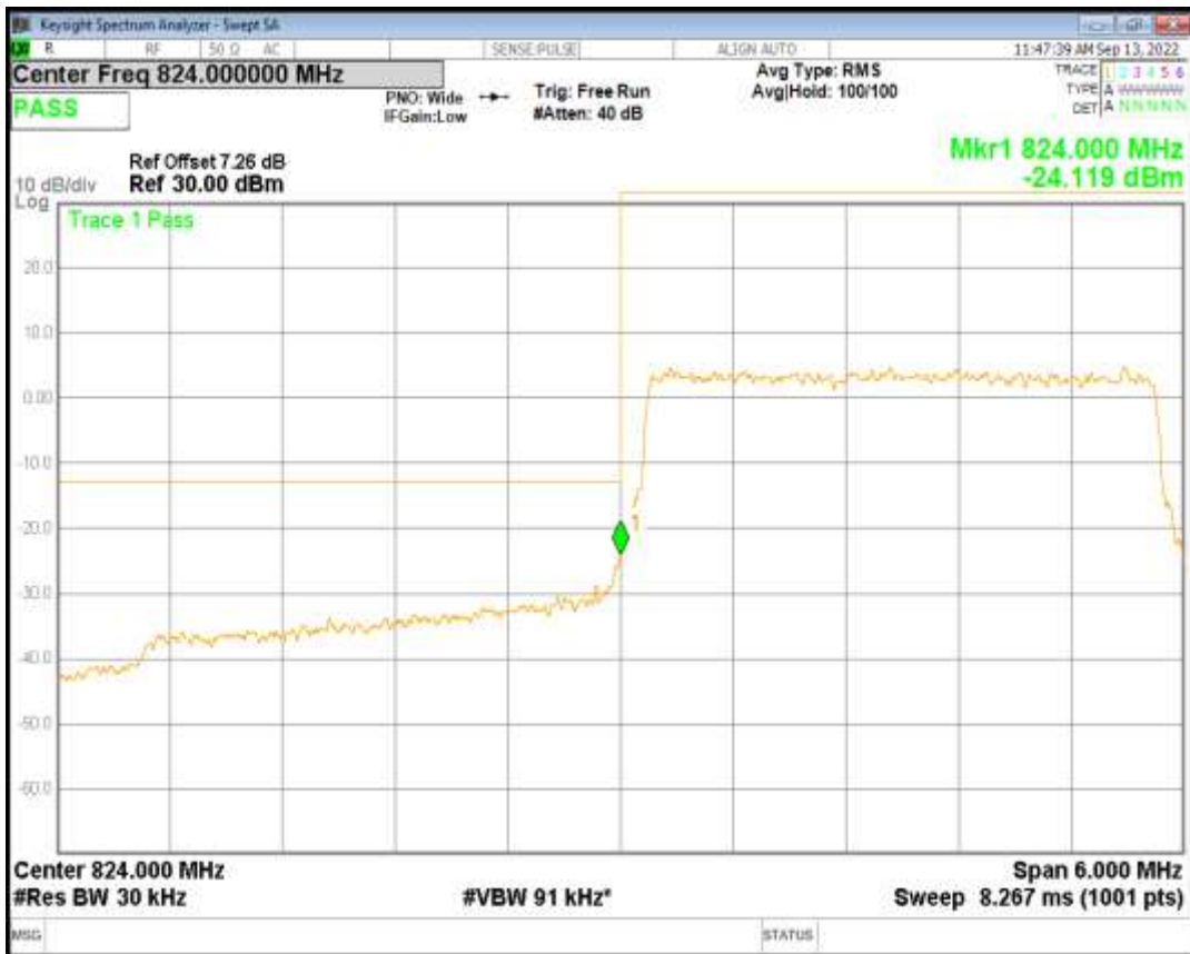
Band26(824-849) QAM16 BW=3MHz Channel=26805 RB Size=15 Position=#0
