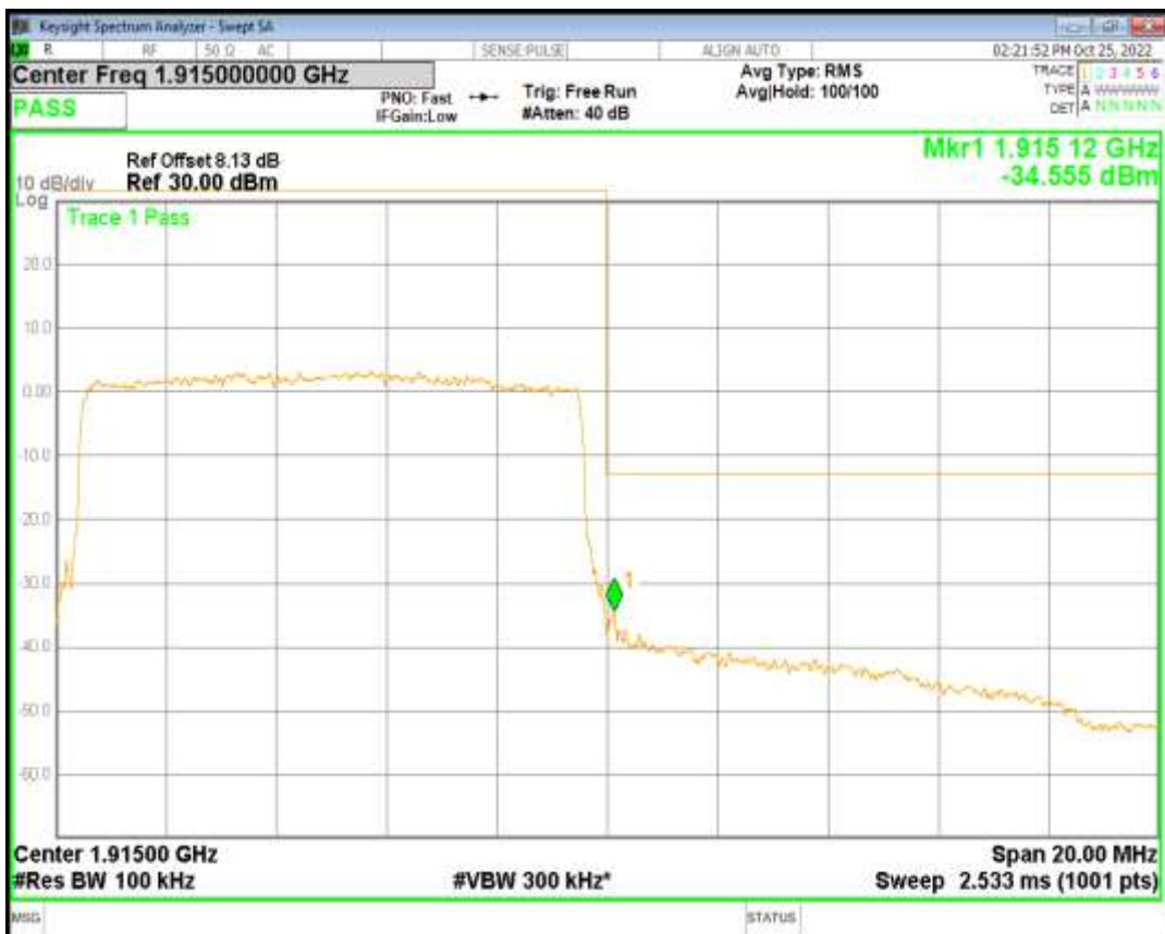
Band25 QAM16 BW=10MHz Channel=26640 RB Size=50 Position=#0
