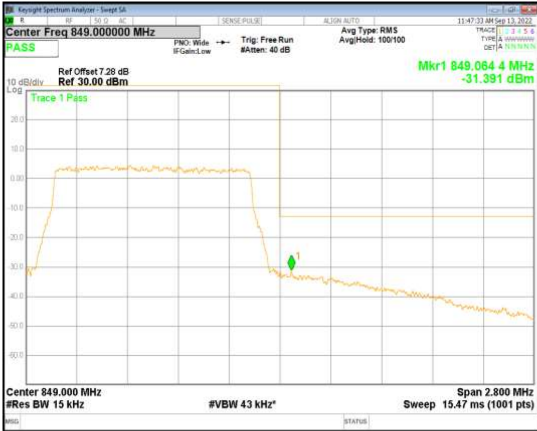
Band26(824-849) QPSK BW=3MHz Channel=26805 RB Size=15 Position=#0
