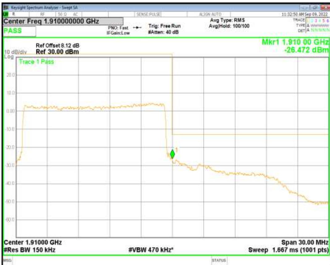
Band2 QAM16 BW=15MHz Channel=19125 RB Size=75 Position=#0
