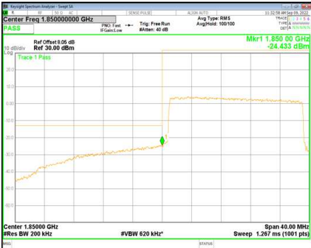
Band2 QAM16 BW=20MHz Channel=18700 RB Size=100 Position=#0
