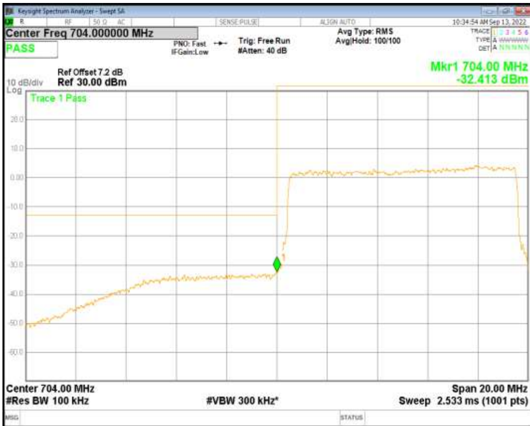
Band17 QPSK BW=10MHz Channel=23800 RB Size=50 Position=#0
