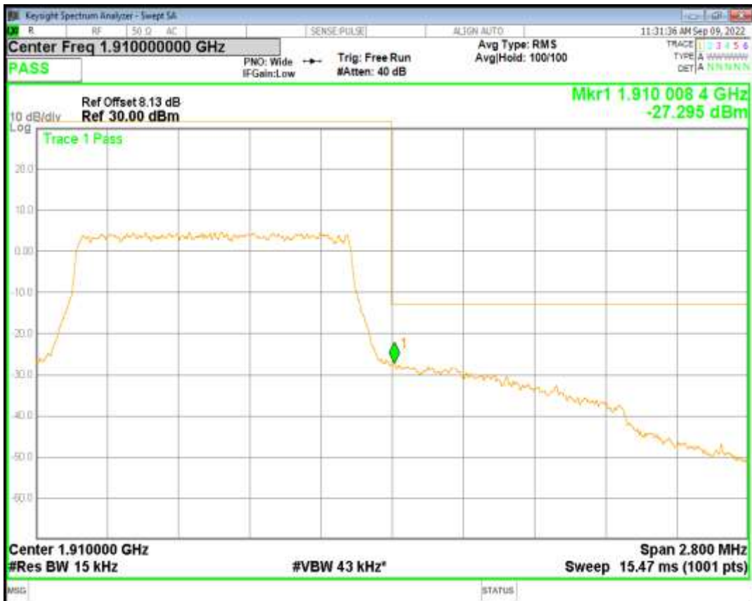
Band2 QAM16 BW=1.4MHz Channel=19193 RB Size=6 Position=#0
