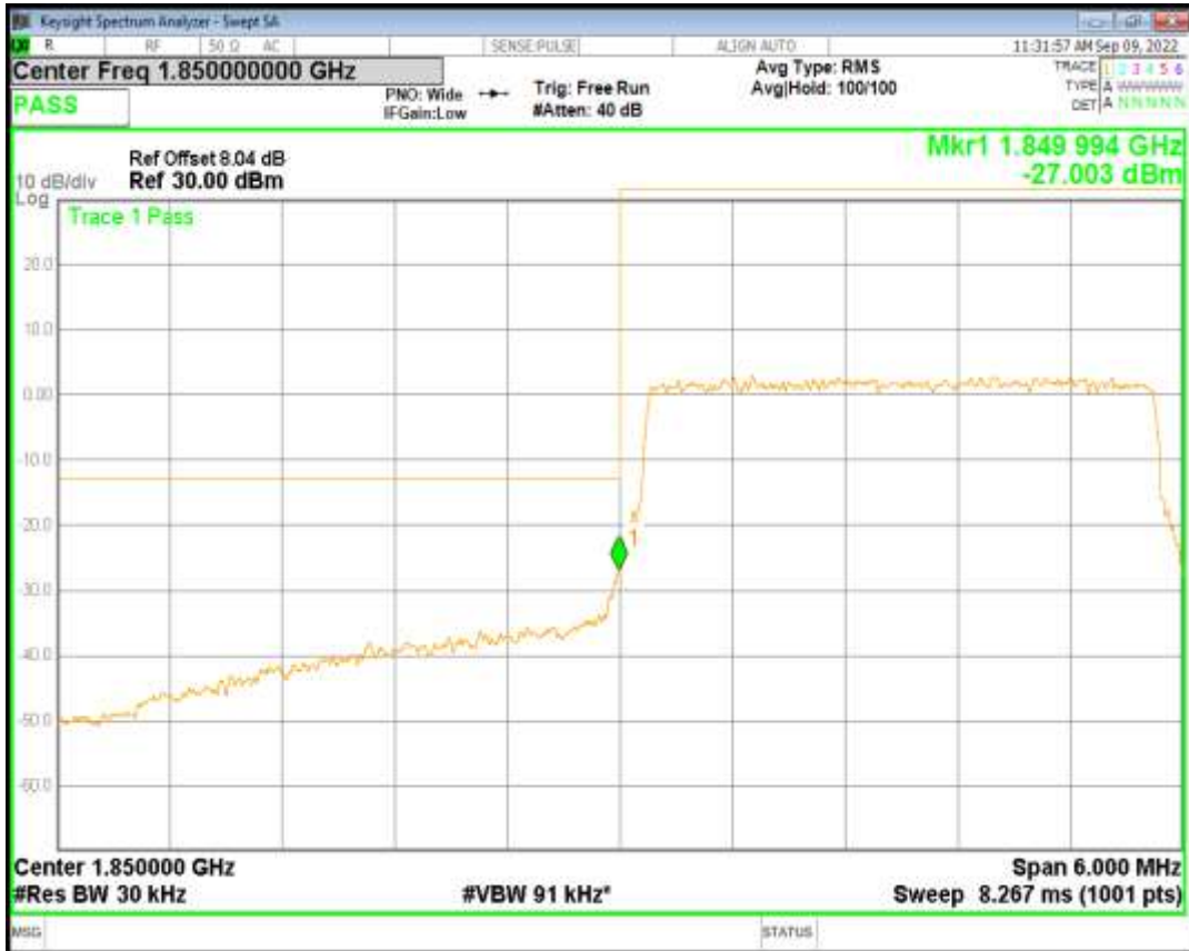
Band2 QPSK BW=3MHz Channel=19185 RB Size=15 Position=#0
