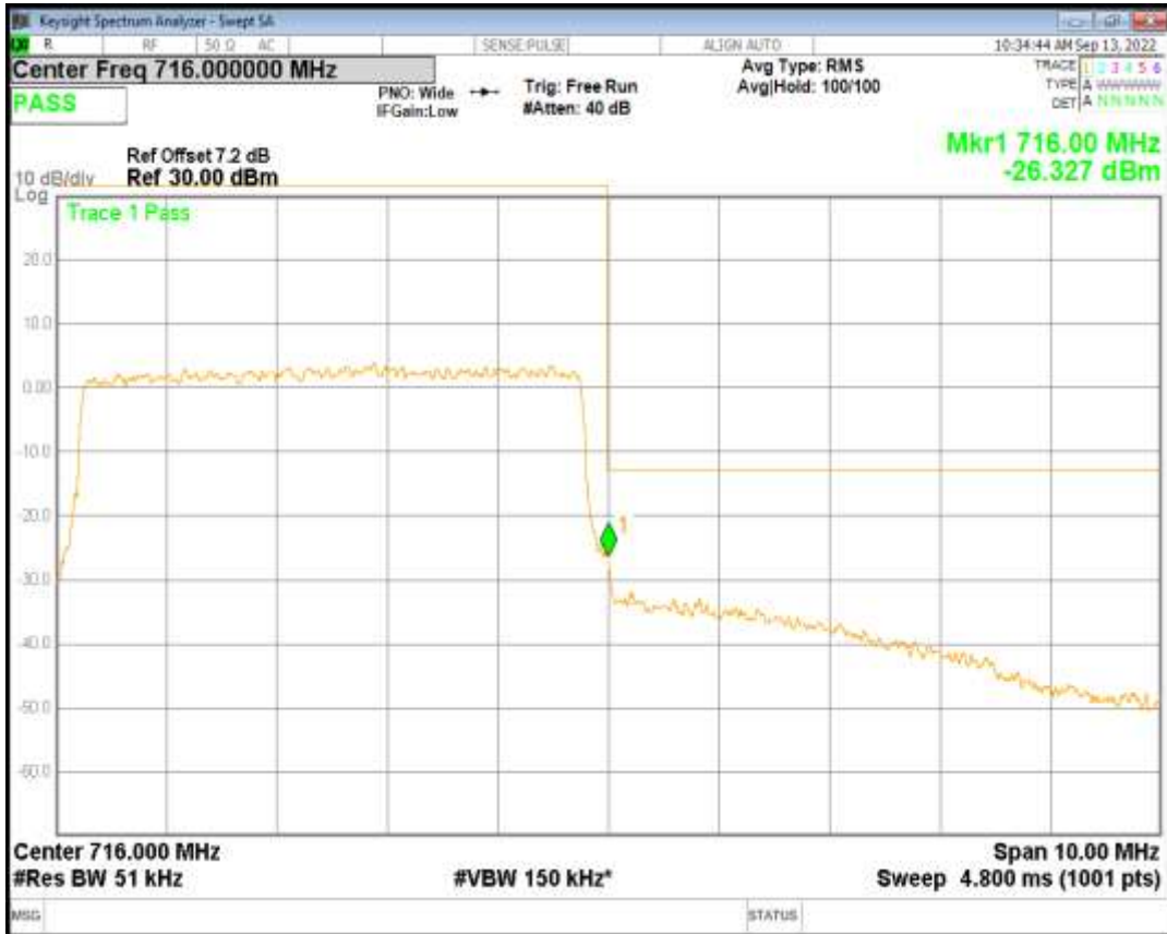
Band17 QPSK BW=10MHz Channel=23780 RB Size=50 Position=#0
