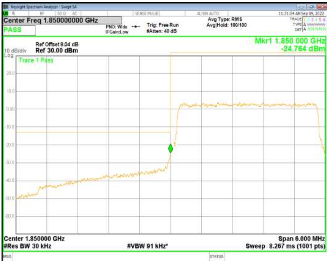
Band2 QAM16 BW=3MHz Channel=18615 RB Size=15 Position=#0
