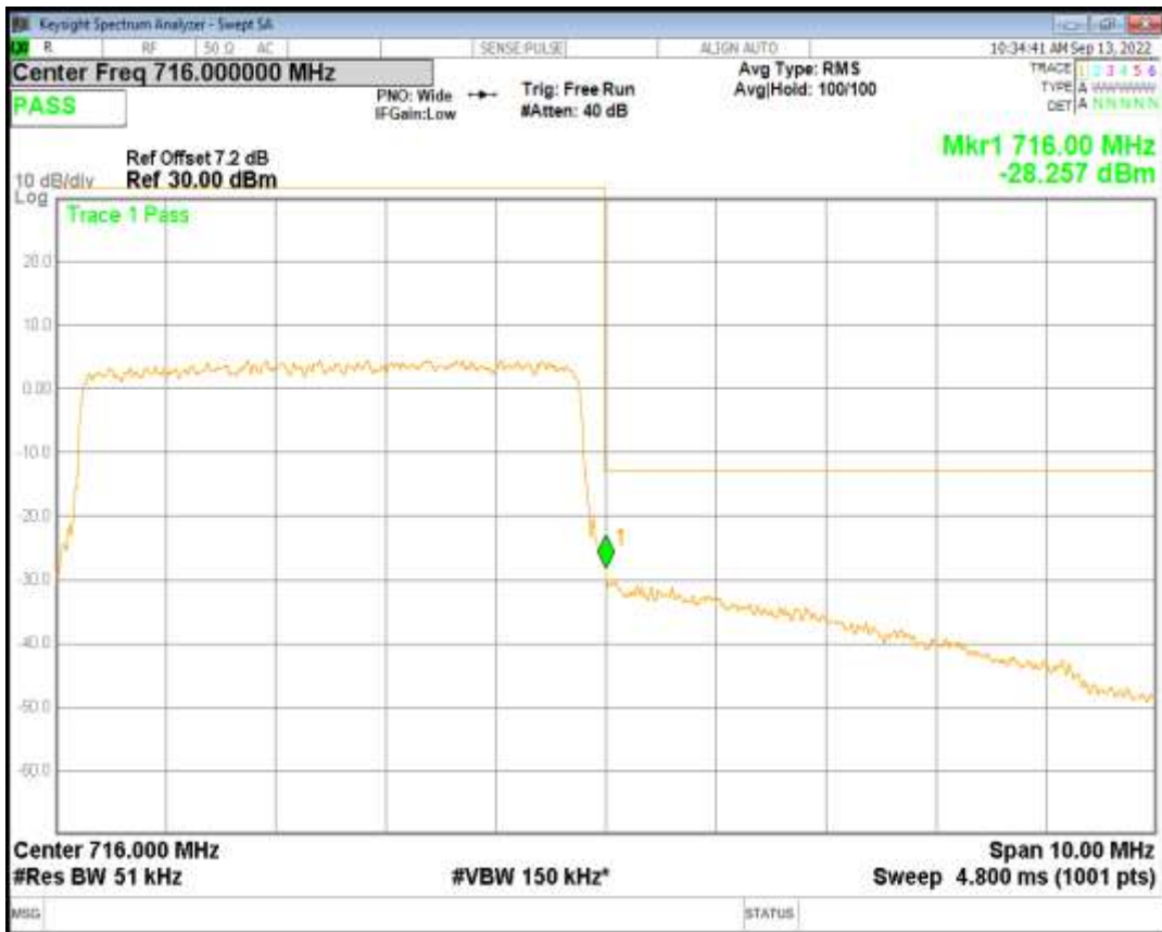
Band17 QAM16 BW=5MHz Channel=23825 RB Size=25 Position=#0
