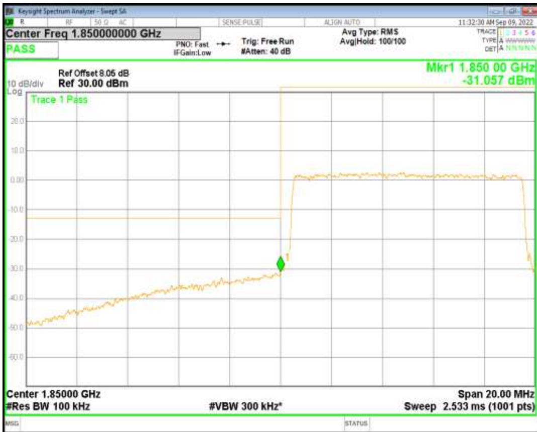
Band2 QPSK BW=10MHz Channel=19150 RB Size=50 Position=#0
