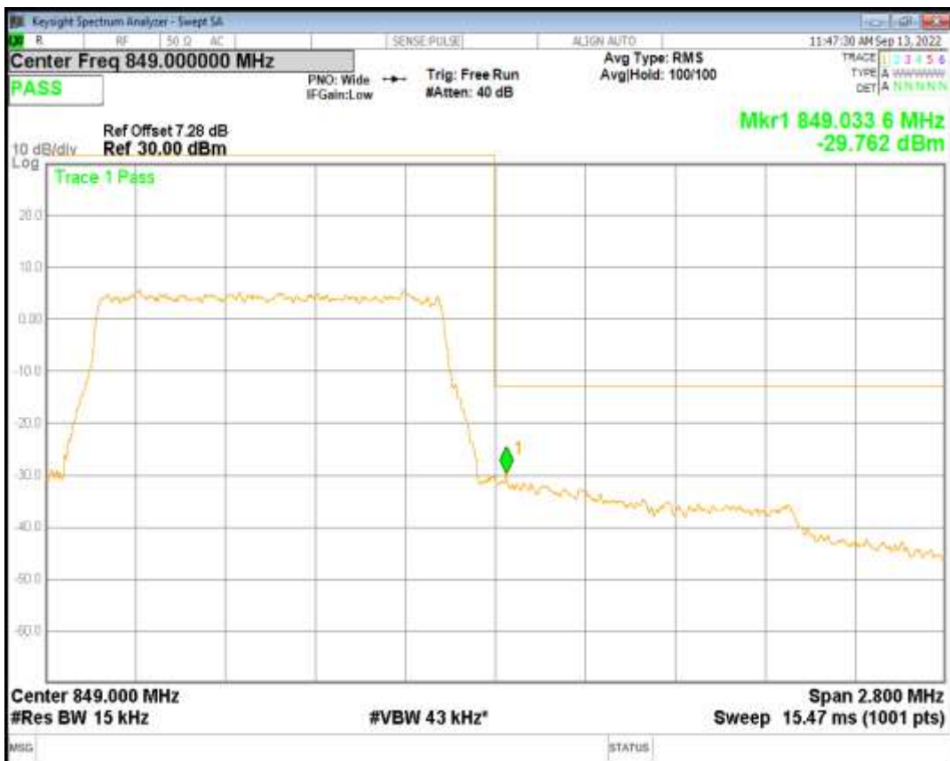
Band26(824-849) QAM16 BW=1.4MHz Channel=27033 RB Size=6 Position=#0
