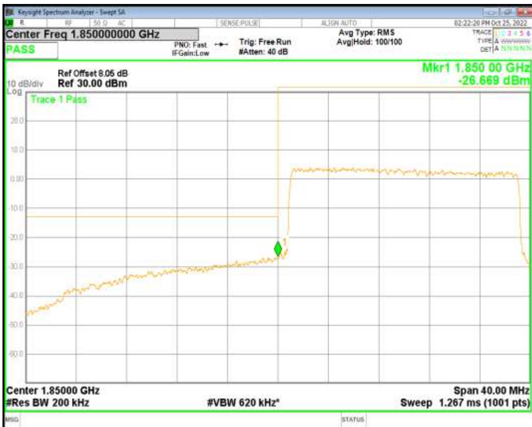
Band25 QAM16 BW=20MHz Channel=26140 RB Size=100 Position=#0
