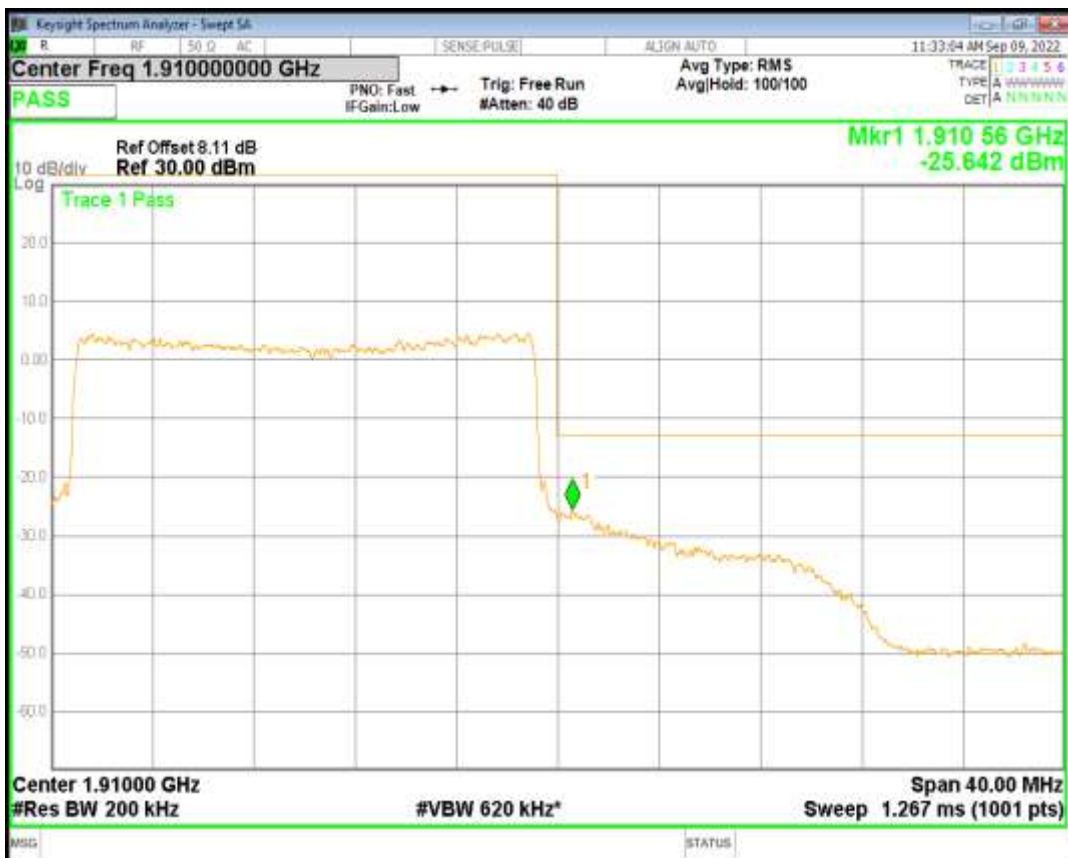
Band2 QAM16 BW=20MHz Channel=19100 RB Size=100 Position=#0
