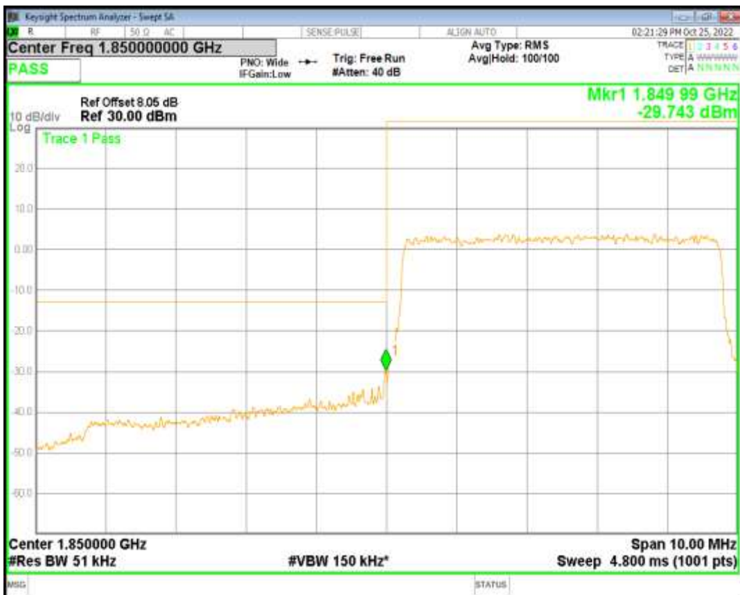
Band25 QAM16 BW=5MHz Channel=26065 RB Size=25 Position=#0
