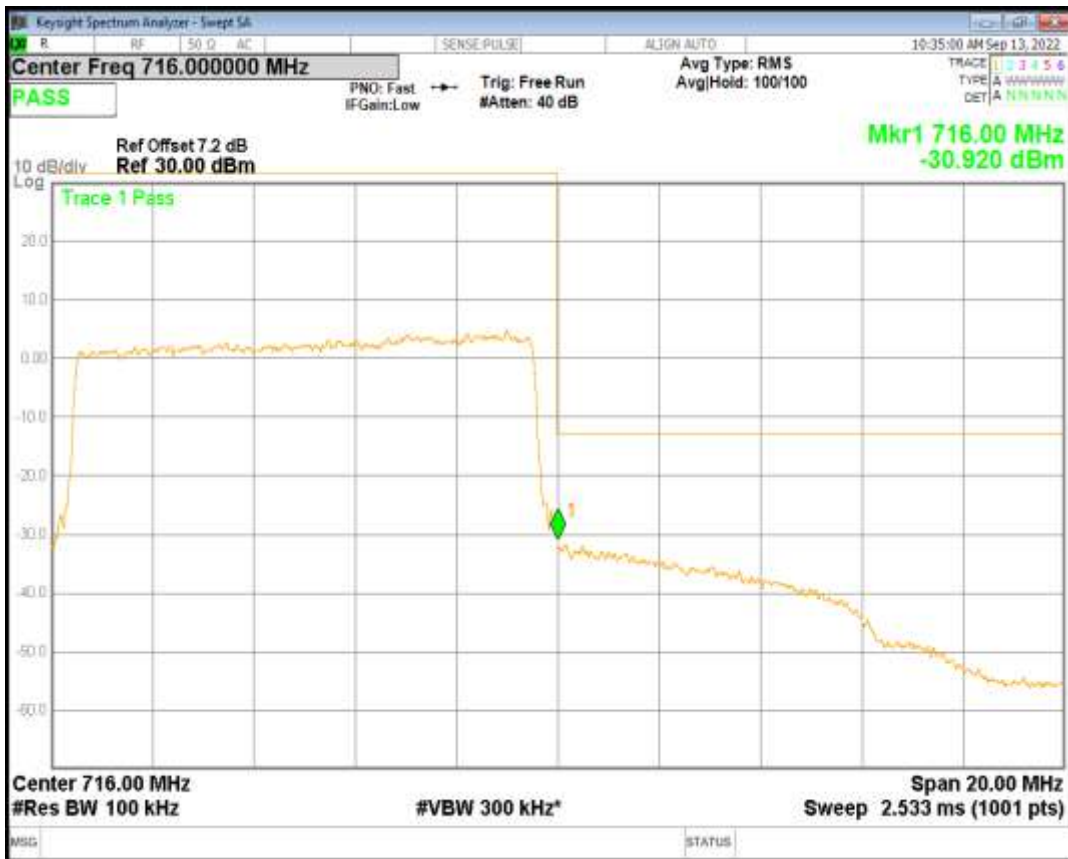
Band2 QPSK BW=1.4MHz Channel=18607 RB Size=6 Position=#0
