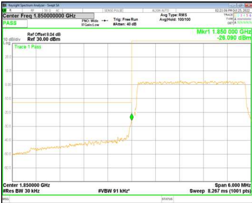
Band25 QPSK BW=3MHz Channel=26675 RB Size=15 Position=#0
