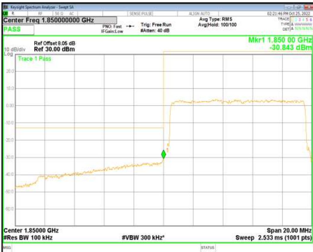
Band25 QAM16 BW=10MHz Channel=26090 RB Size=50 Position=#0
