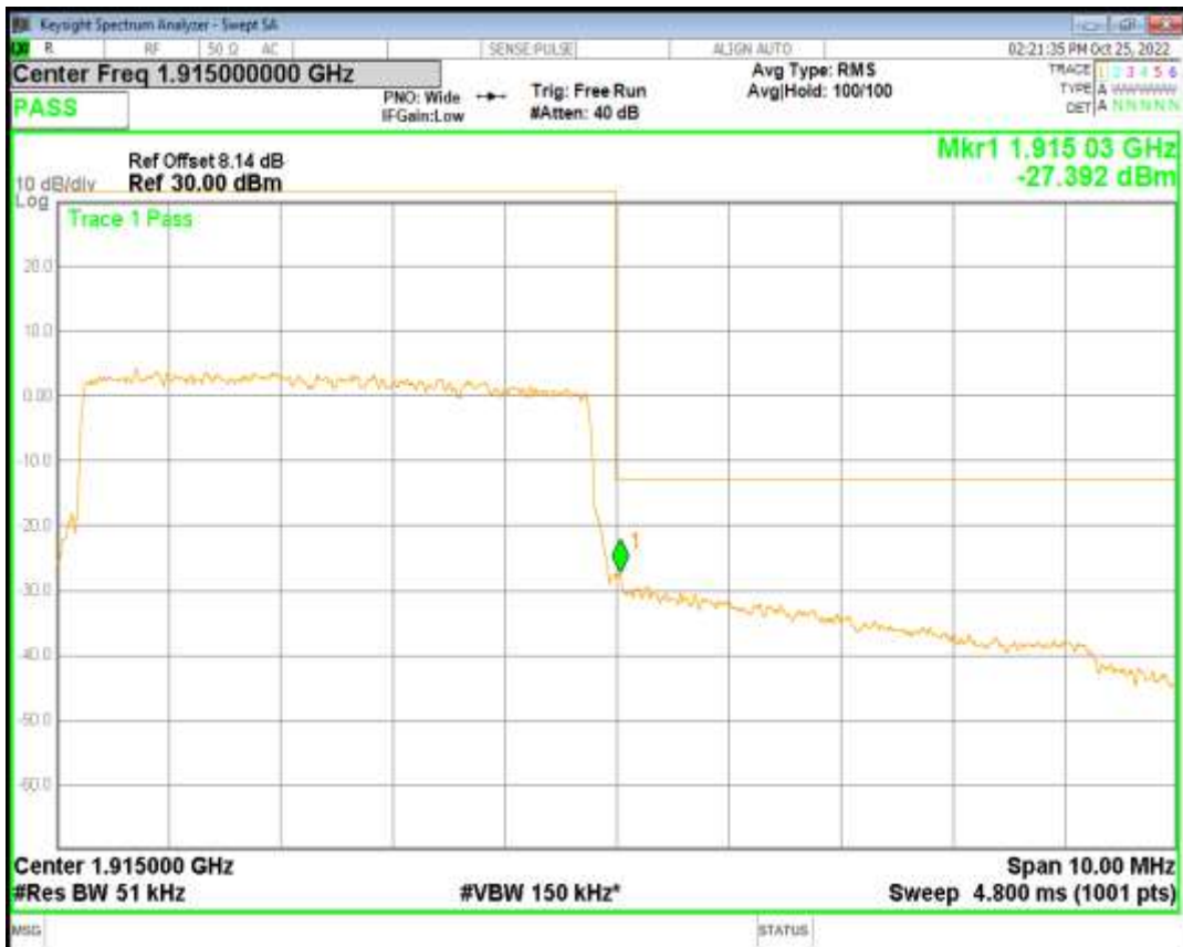
Band25 QAM16 BW=5MHz Channel=26665 RB Size=25 Position=#0
