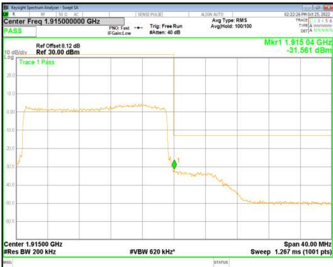
Band25 QAM16 BW=20MHz Channel=26590 RB Size=100 Position=#0
