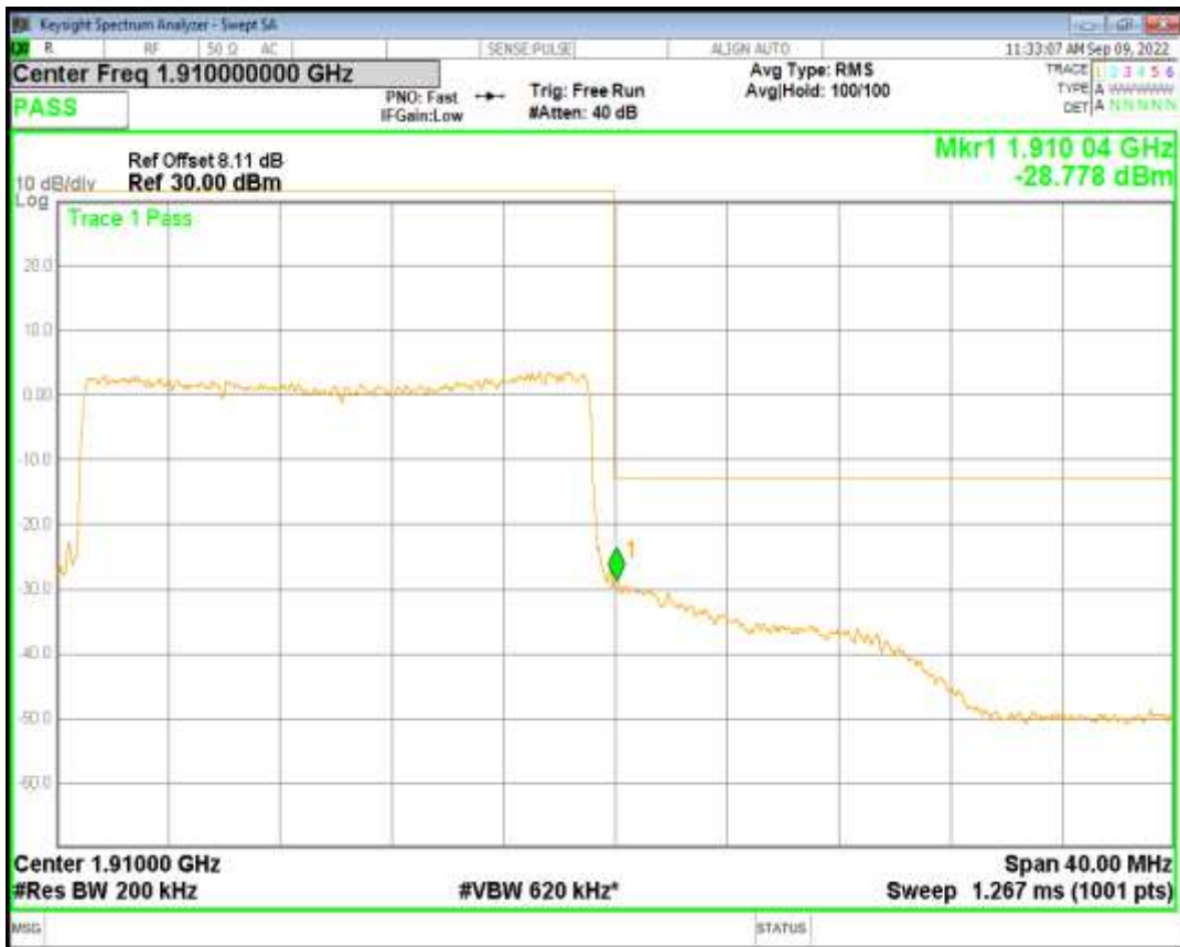
Band25 QPSK BW=1.4MHz Channel=26047 RB Size=6 Position=#0
