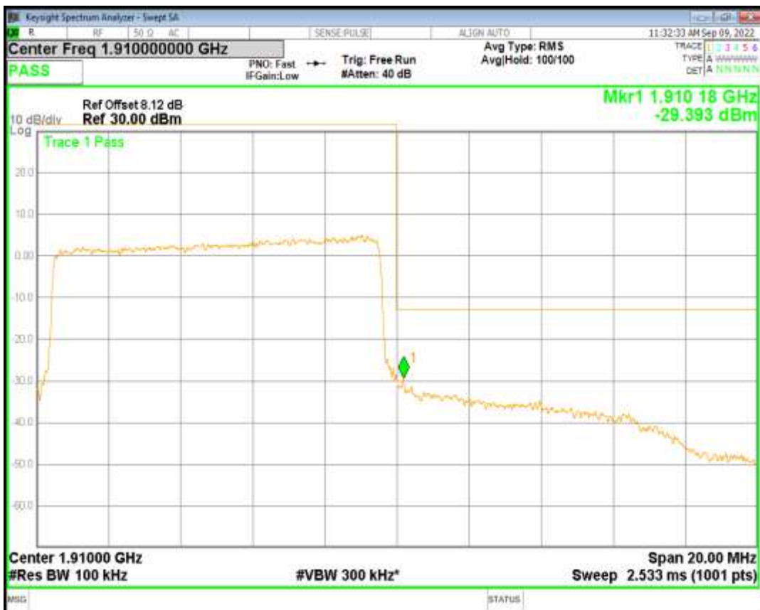
Band2 QAM16 BW=10MHz Channel=19150 RB Size=50 Position=#0
