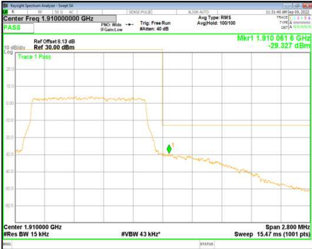
Band2 QPSK BW=3MHz Channel=18615 RB Size=15 Position=#0
