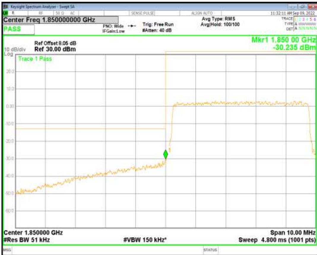
Band2 QPSK BW=5MHz Channel=19175 RB Size=25 Position=#0
