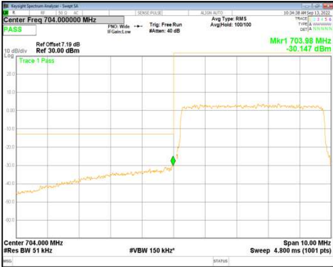
Band17 QPSK BW=5MHz Channel=23825 RB Size=25 Position=#0
