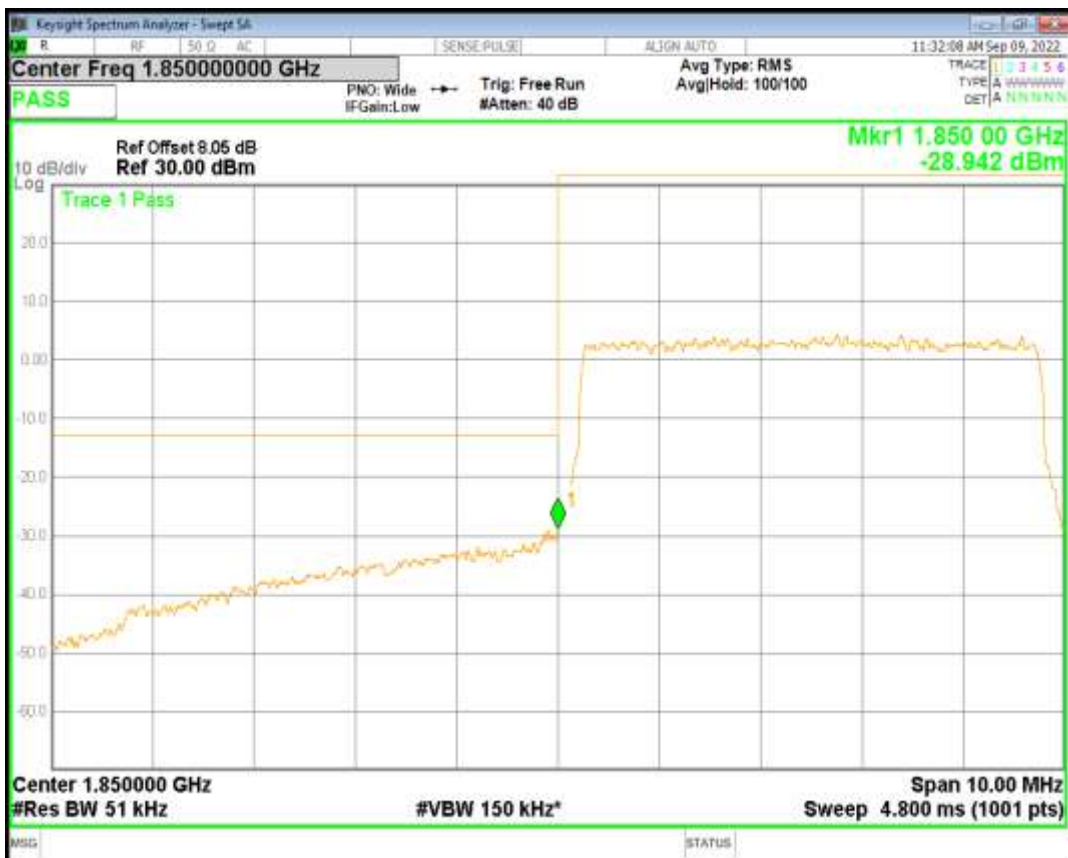
Band2 QAM16 BW=5MHz Channel=18625 RB Size=25 Position=#0
