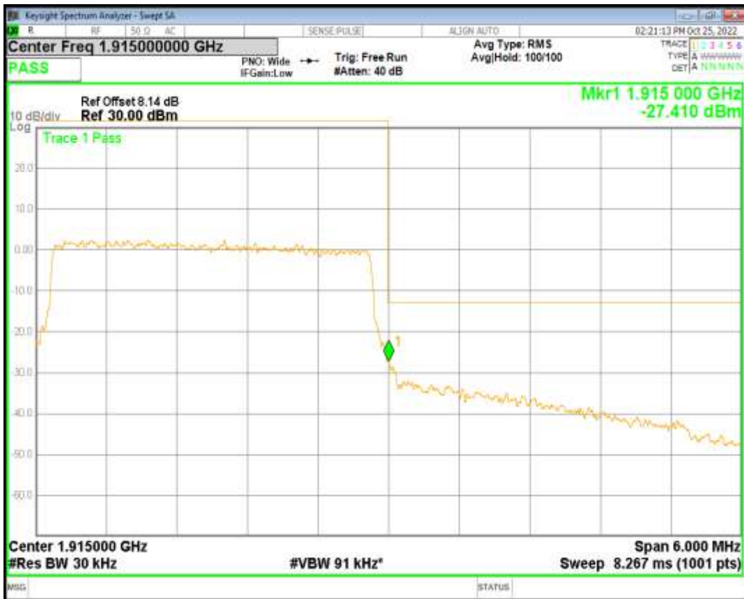
Band25 QPSK BW=5MHz Channel=26065 RB Size=25 Position=#0
