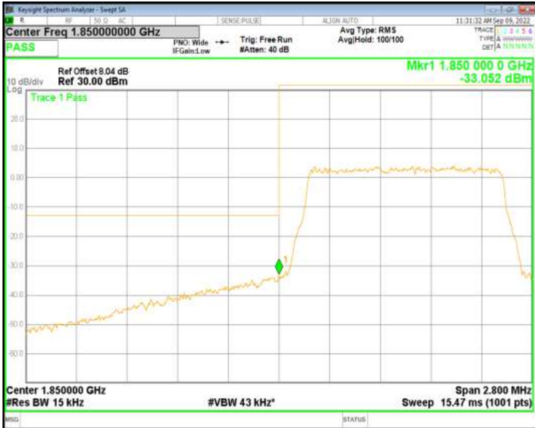
Band2 QPSK BW=1.4MHz Channel=19193 RB Size=6 Position=#0
