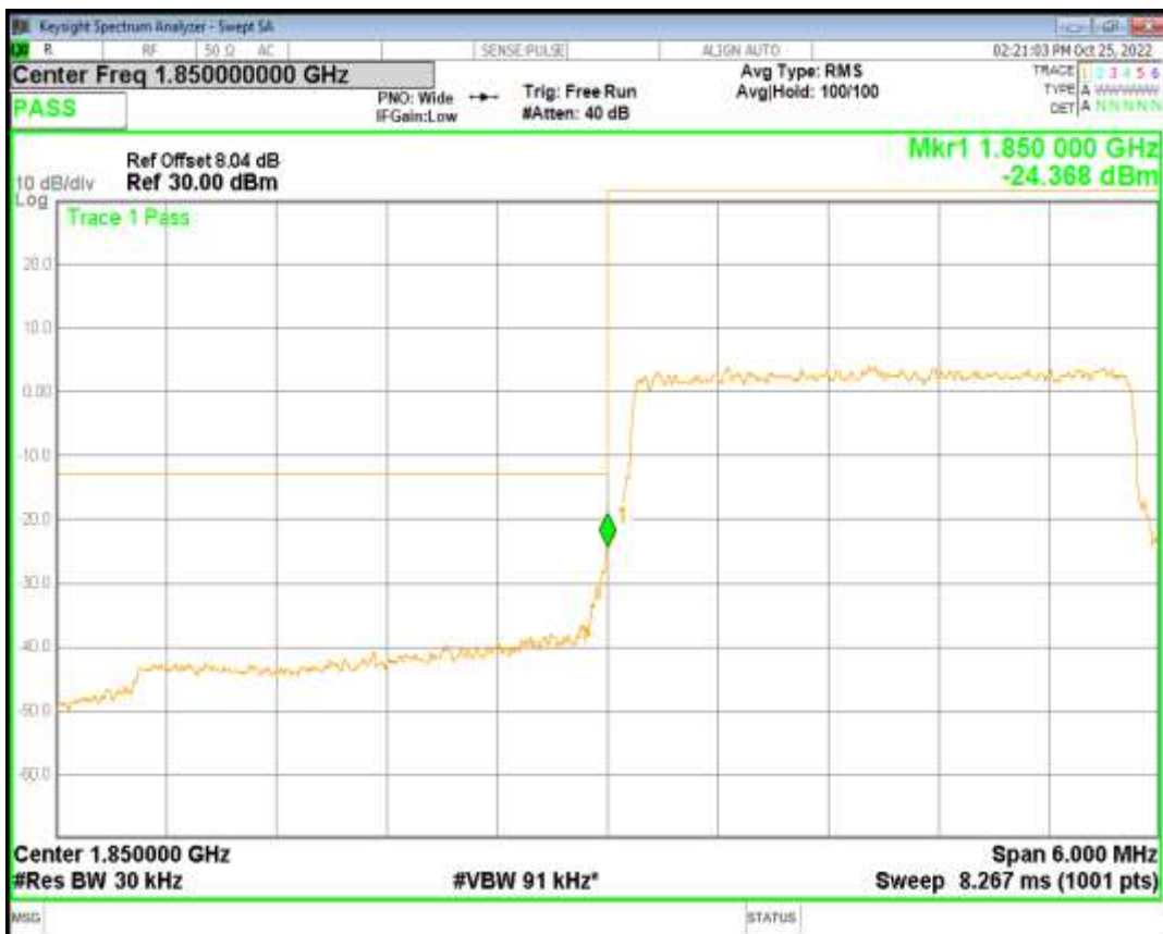
Band25 QAM16 BW=3MHz Channel=26055 RB Size=15 Position=#0
