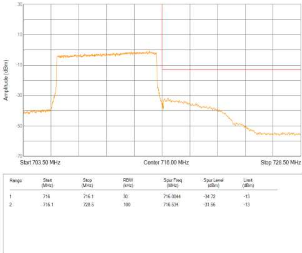
Band17 QPSK BW=5MHz Channel=23755 RB Size=25 Position=#0
