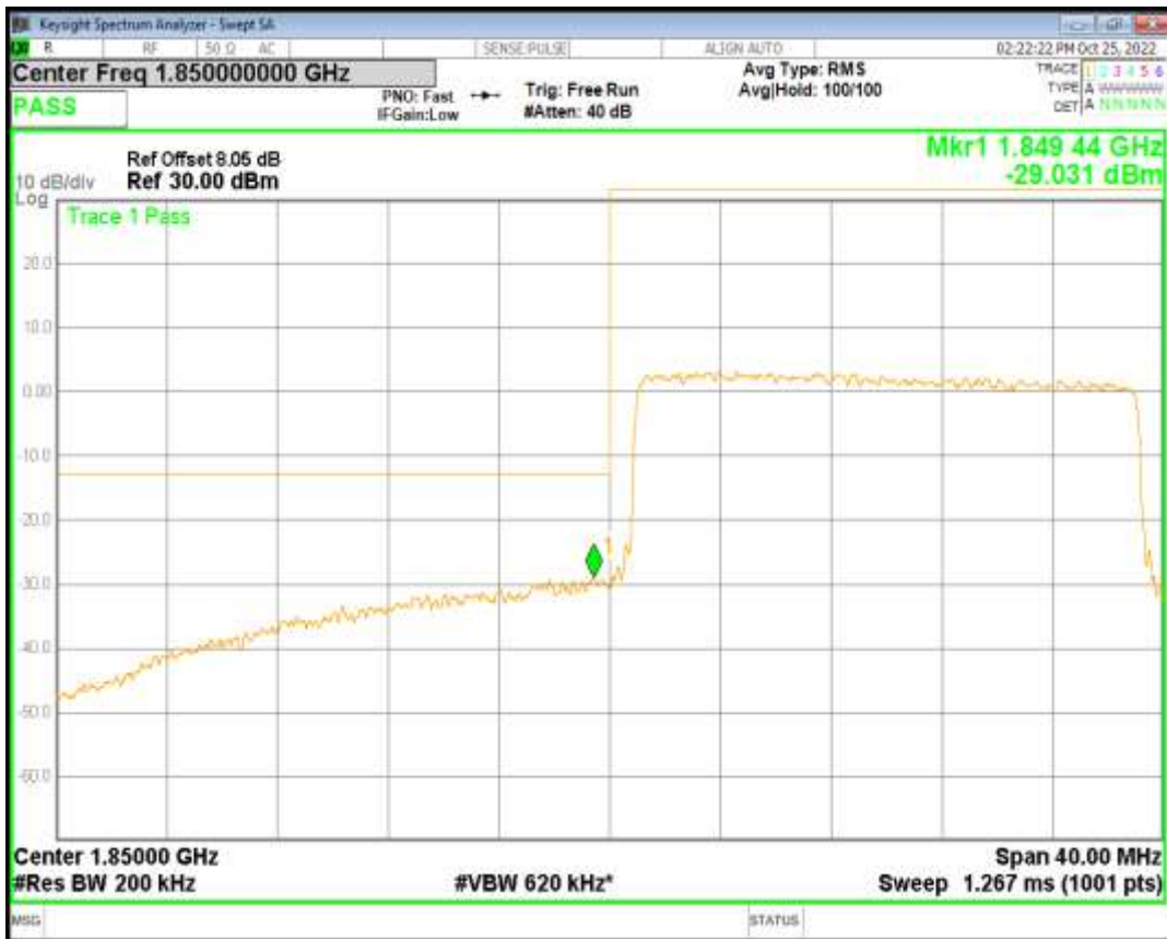
Band25 QPSK BW=20MHz Channel=26590 RB Size=100 Position=#0
