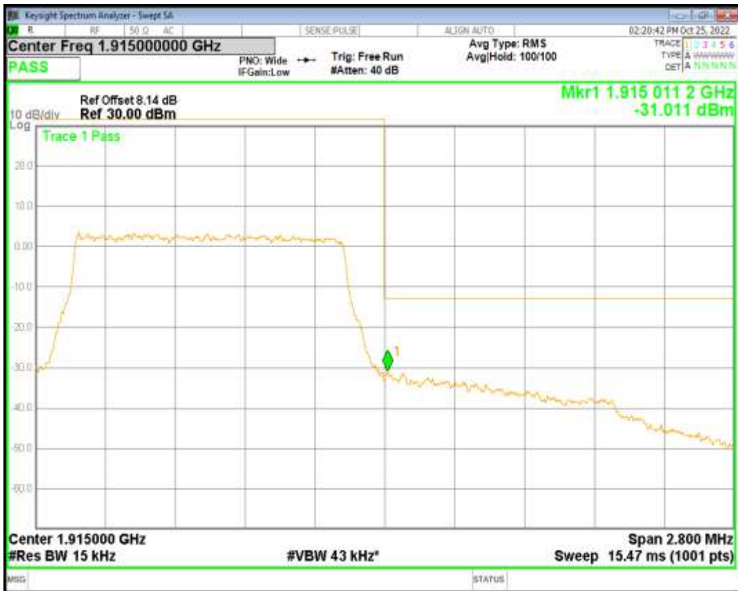
Band25 QAM16 BW=1.4MHz Channel=26683 RB Size=6 Position=#0
