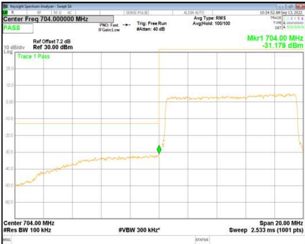
Band17 QAM16 BW=10MHz Channel=23780 RB Size=50 Position=#0
