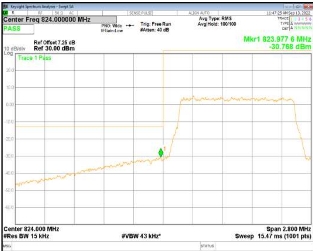
Band26(824-849) QPSK BW=1.4MHz Channel=27033 RB Size=6 Position=#0
