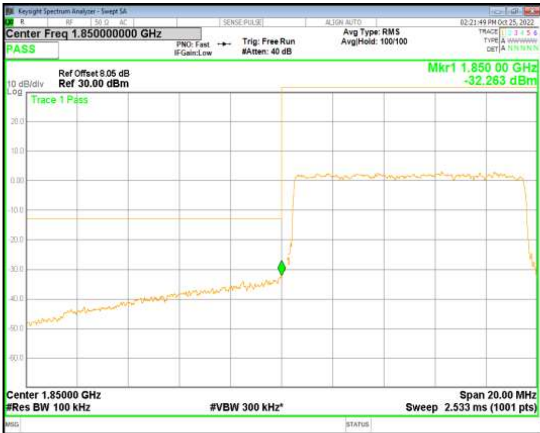
Band25 QPSK BW=10MHz Channel=26640 RB Size=50 Position=#0
