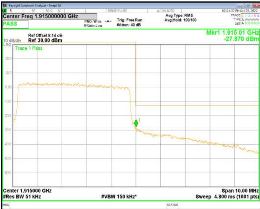
Band25 QPSK BW=10MHz Channel=26090 RB Size=50 Position=#0
