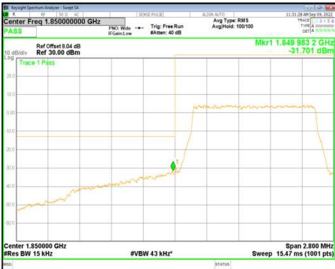
Band2 QAM16 BW=1.4MHz Channel=18607 RB Size=6 Position=#0
