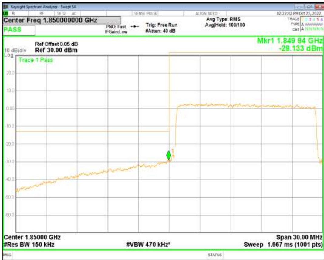
Band25 QPSK BW=15MHz Channel=26615 RB Size=75 Position=#0
