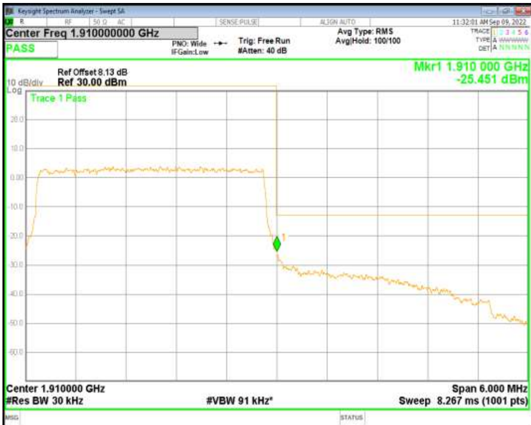
Band2 QAM16 BW=3MHz Channel=19185 RB Size=15 Position=#0
