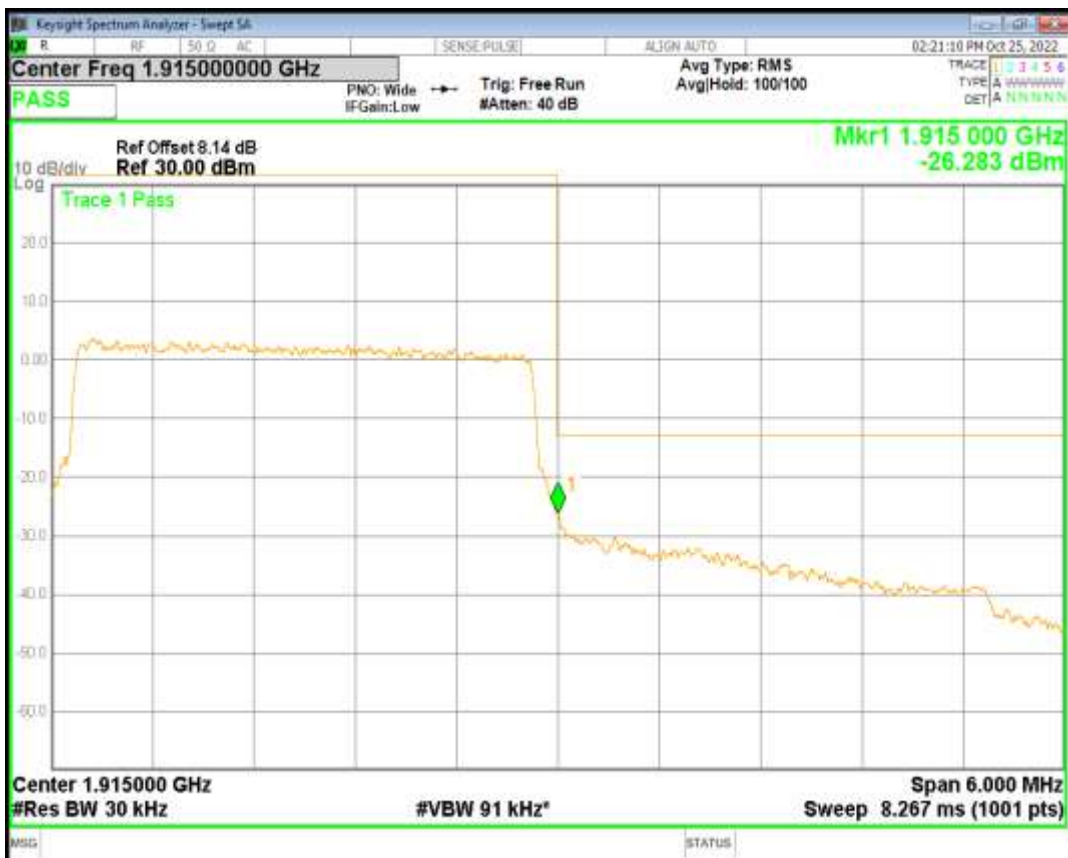
Band25 QAM16 BW=3MHz Channel=26675 RB Size=15 Position=#0
