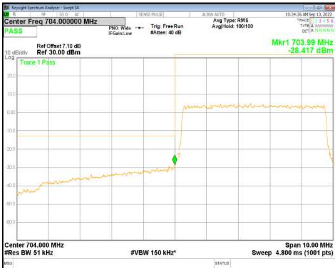
Band17 QAM16 BW=5MHz Channel=23755 RB Size=25 Position=#0
