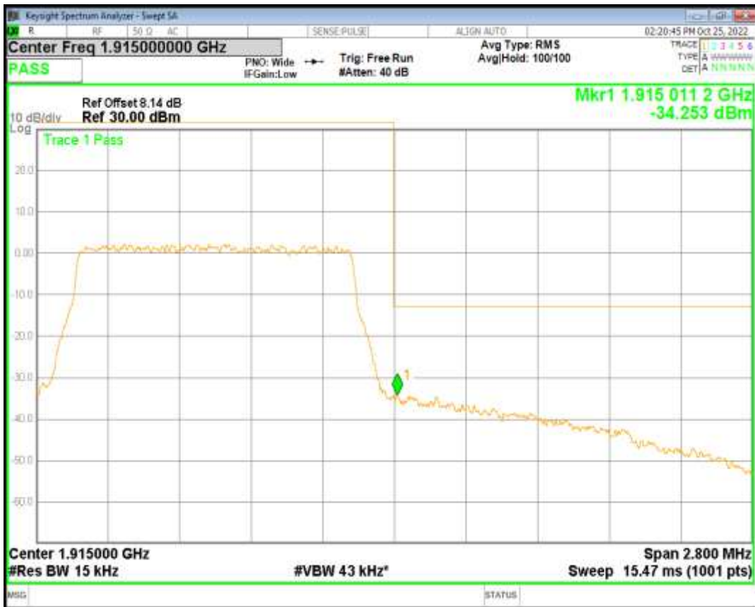
Band25 QPSK BW=3MHz Channel=26055 RB Size=15 Position=#0
