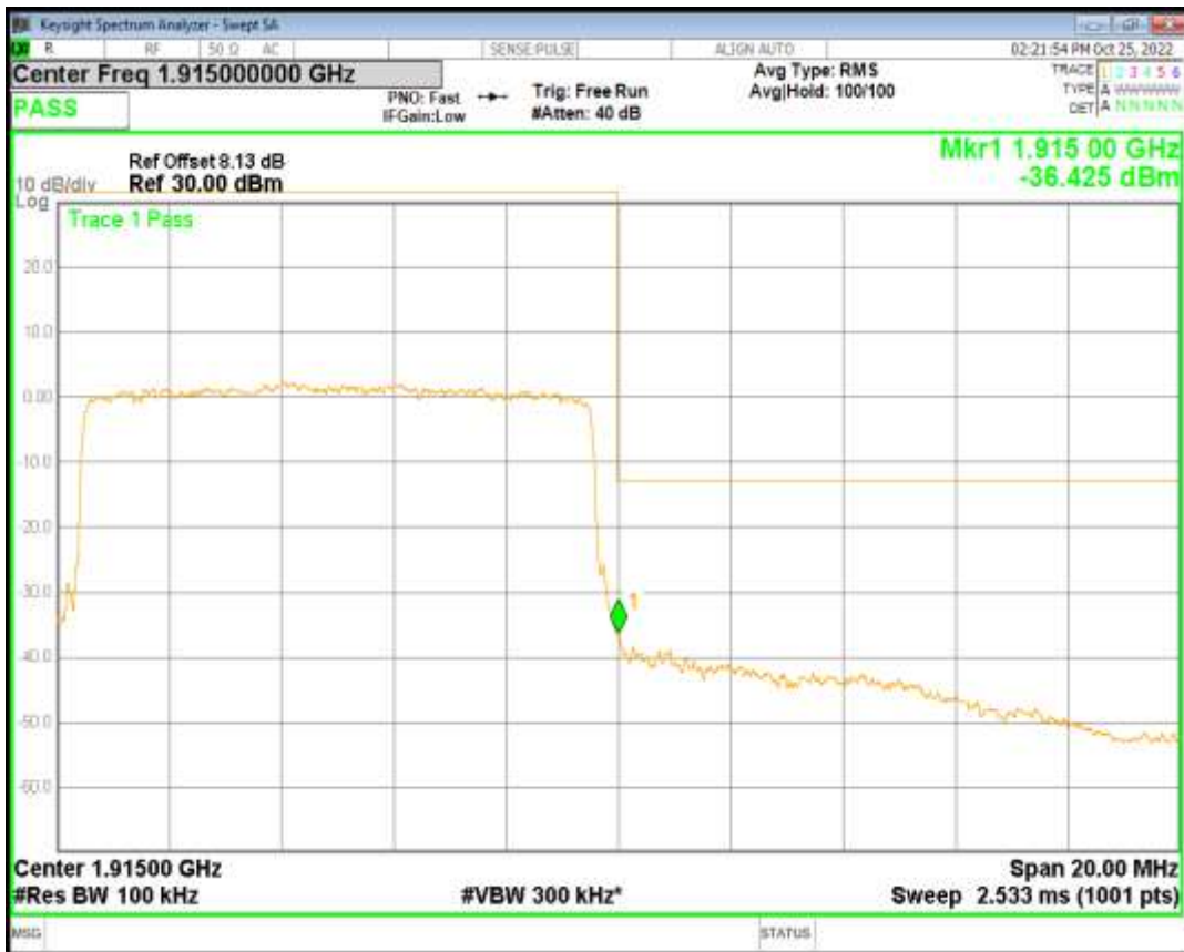
Band25 QPSK BW=15MHz Channel=26115 RB Size=75 Position=#0
