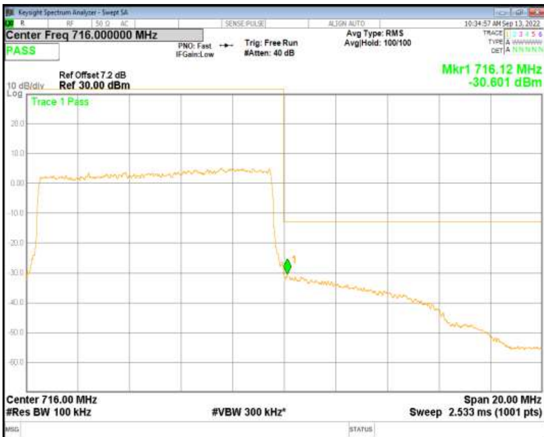
Band17 QAM16 BW=10MHz Channel=23800 RB Size=50 Position=#0
