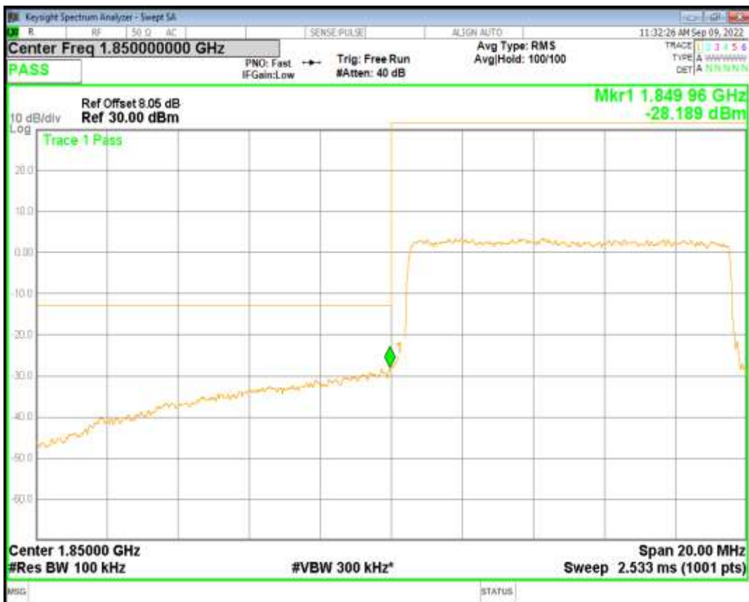
Band2 QAM16 BW=10MHz Channel=18650 RB Size=50 Position=#0
