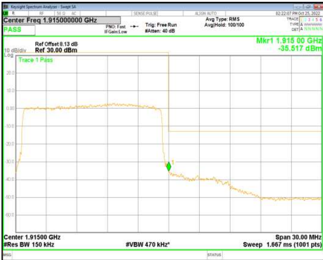
Band25 QPSK BW=20MHz Channel=26140 RB Size=100 Position=#0
