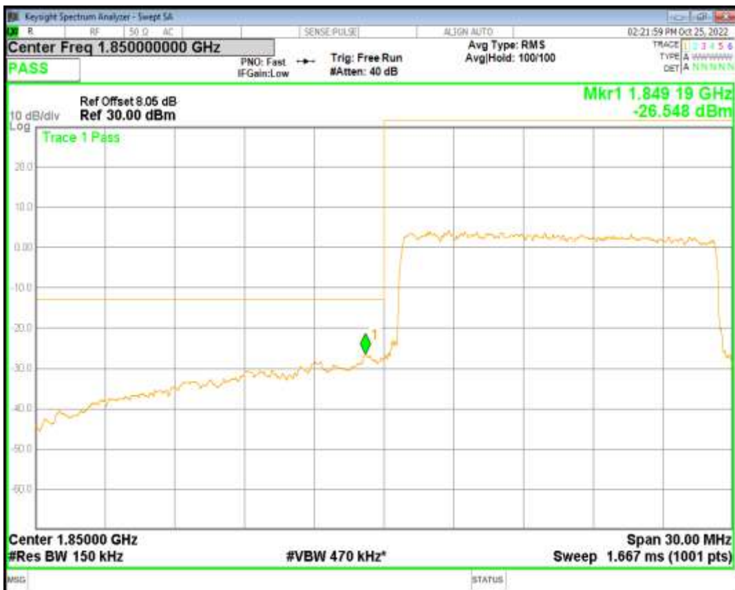
Band25 QAM16 BW=15MHz Channel=26115 RB Size=75 Position=#0
