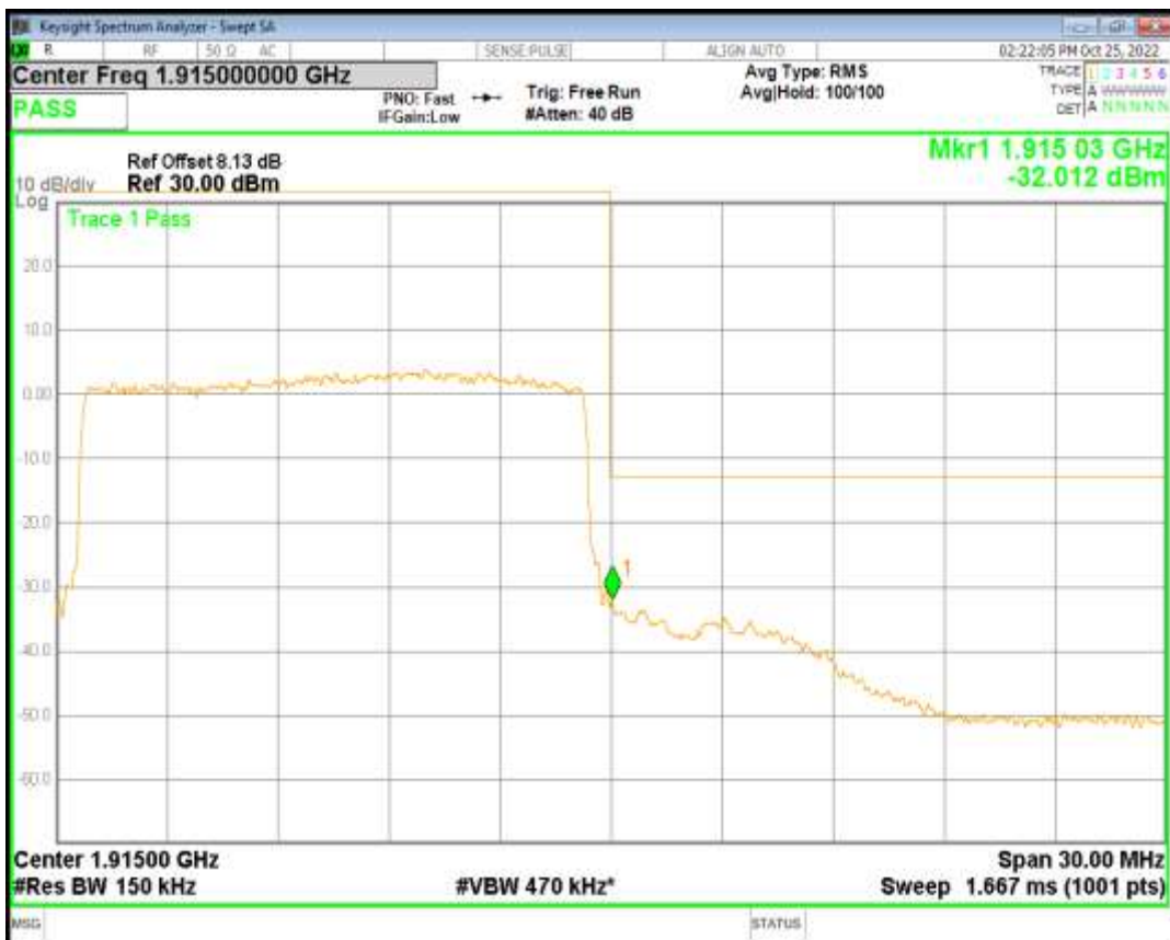
Band25 QAM16 BW=15MHz Channel=26615 RB Size=75 Position=#0
