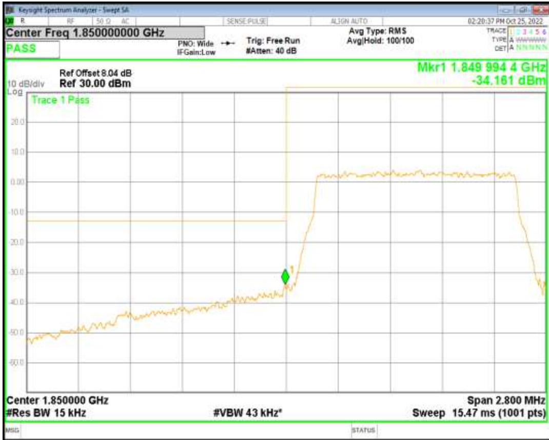
Band25 QPSK BW=1.4MHz Channel=26683 RB Size=6 Position=#0
