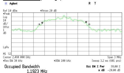
Transmit Freq Error -71.036 kHz x dB Bandwidth 1.216 MHz
