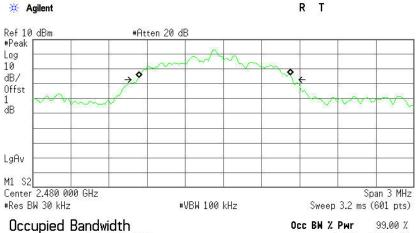
Occupied Bandwidth 1.1923 MHz Occ BW % Pwr 99.00 % x dB -20.00 dB
