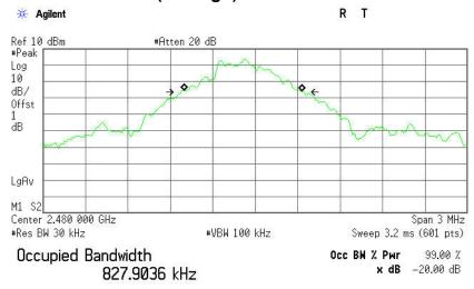
Transmit Freq Error -83.615 kHz x dB Bandwidth 868.926 kHz
