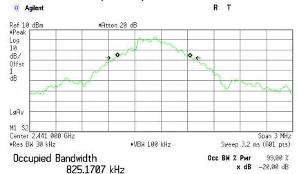
Transmit Freq Error -82.162 kHz x dB Bandwidth 870.372 kHz
