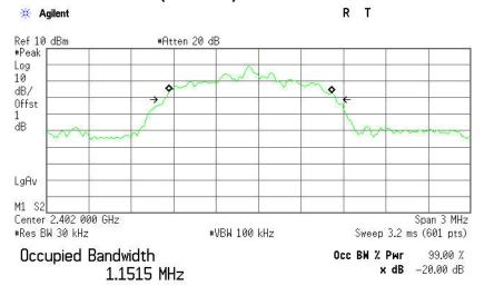
Transmit Freq Error -60.149 kHz x dB Bandwidth 1.213 MHz
