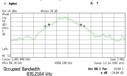
Transmit Freq Error -75.417 kHz x dB Bandwidth 876.560 kHz
