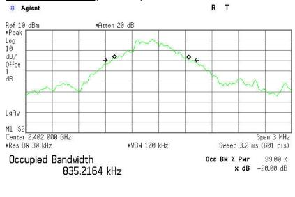
Transmit Freq Error -75.417 kHz x dB Bandwidth 876.560 kHz
