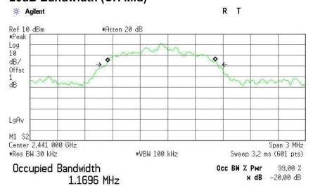
Transmit Freq Error -69.682 kHz x dB Bandwidth 1.216 MHz
