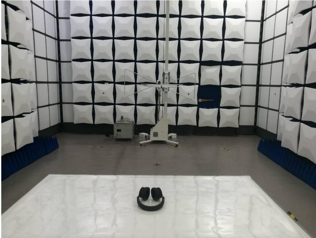
FCC RADIATED EMISSION TEST SETUP
