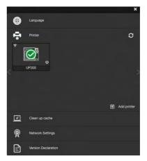
Using the touchscreen on the UP300D to setup the Wifi connection:
