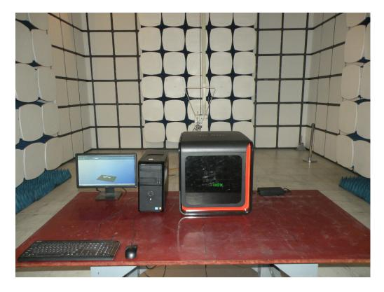
Radiated Emission Test Setup in Chamber
