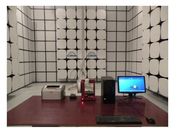
Radiated Emission Test Setup in Chamber
